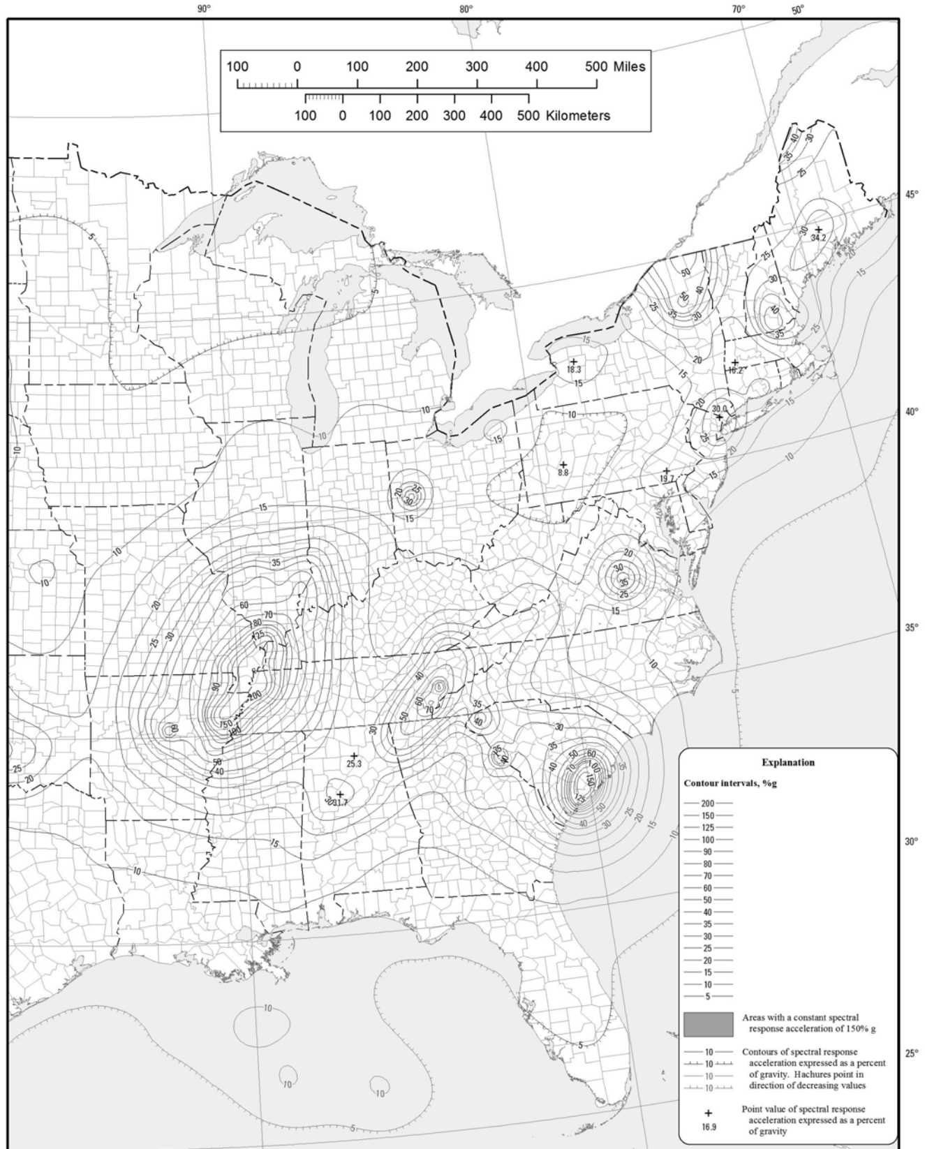
FIGURE 1613.2.1(2) RISK-TARGETED MAXIMUM CONSIDERED EARTHQUAKE (MCE R ) GROUND MOTION RESPONSE ACCELERATIONS FOR THE CONTIGUOUS UNITED STATES OF 0.2-SECOND SPECTRAL RESPONSE ACCELERATION (5% OF CRITICAL DAMPING)
