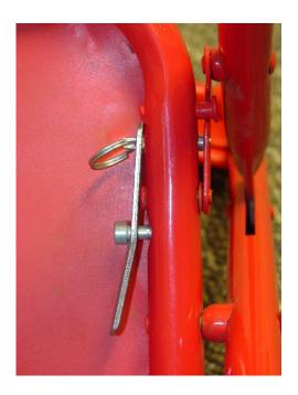
Figure 2. Spring-Loaded Locking Pin Mechanism
