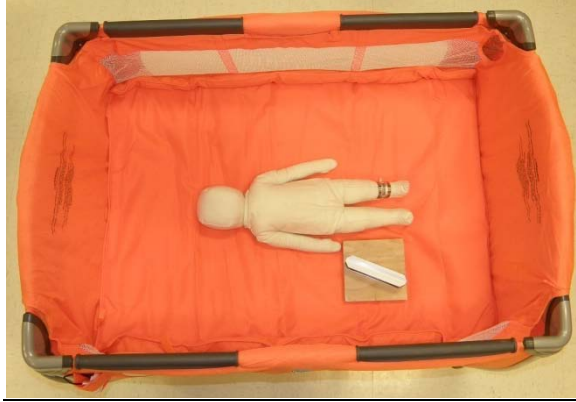
FIG. A1.41 Bassinet/cradle accessory sleep surface test angle measurement.
