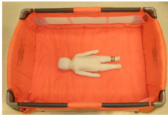
FIG. A1.40 Infant CAMI dummy positioned for bassinet/cradle accessory sleep surface test.
