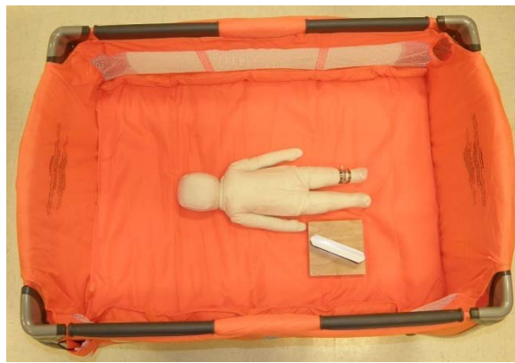
Figure D. Bassinet/cradle accessory sleep surface test angle measurement.
