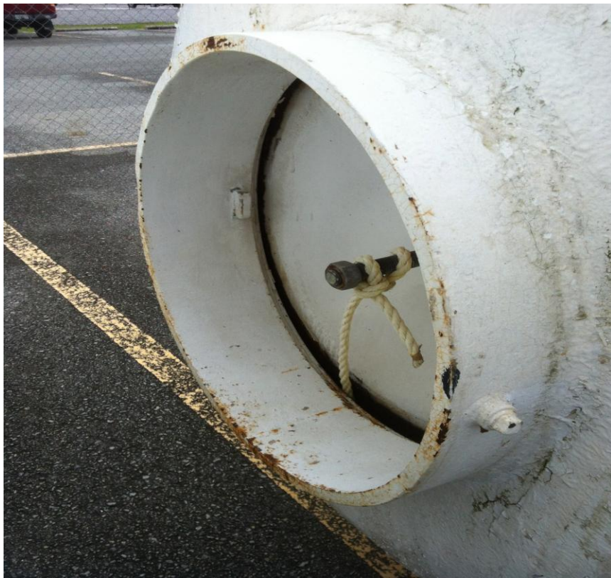
Two random surface diving deck chambers showing different man-way designs
