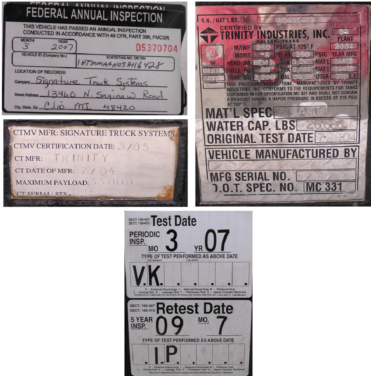
Figure 1. Data and certification information for International truck and Trinity cargo tank.
