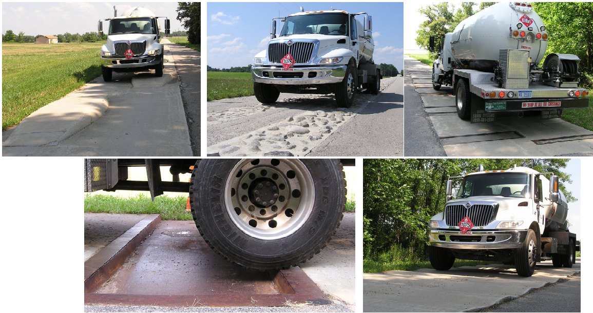
Figure 15. TRC Durability Course Loadings, clockwise from top left: Frame Twist Humps, Cobblestones, Random Chuckholes, Washboard, Deep Chuckholes.
