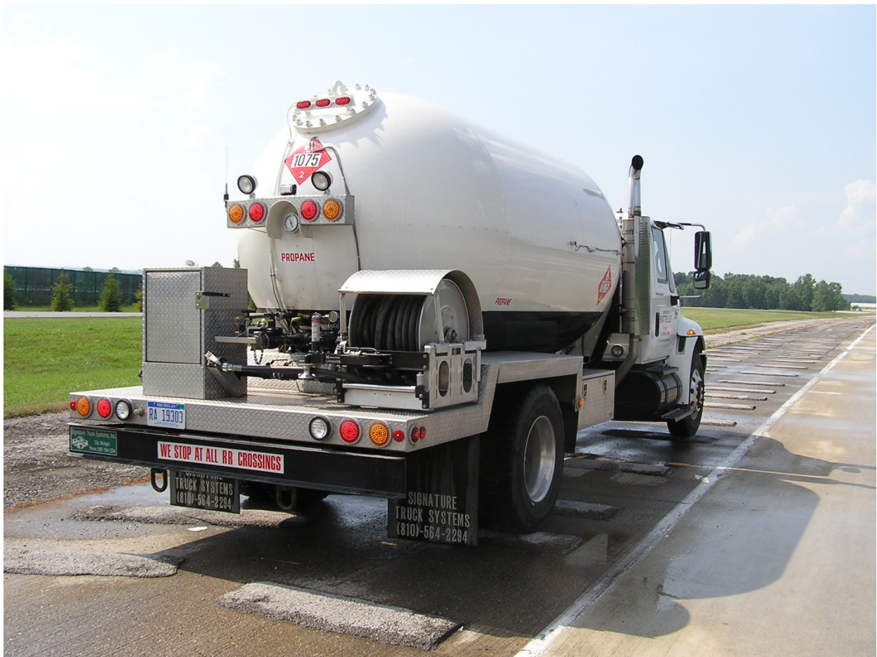
Figure 3. Propane truck used to acquire the over-the-road strain data – rear-quarter view.
