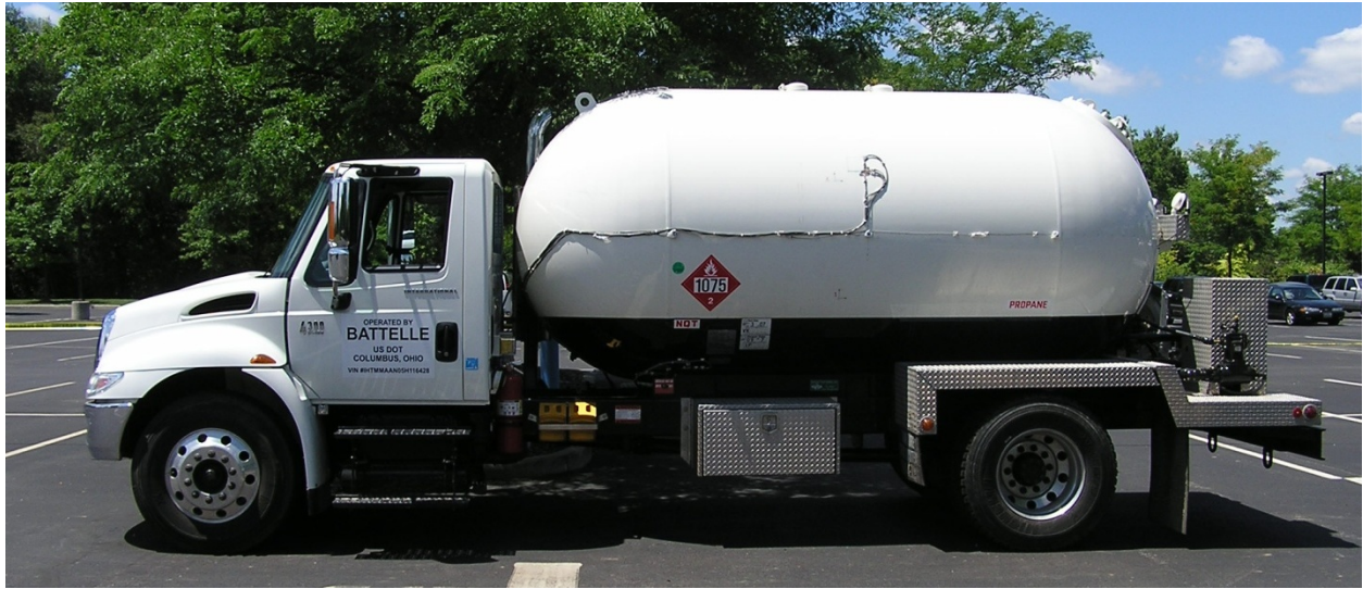
Figure 2. Propane truck used to acquire the over-the-road strain data – side view.
