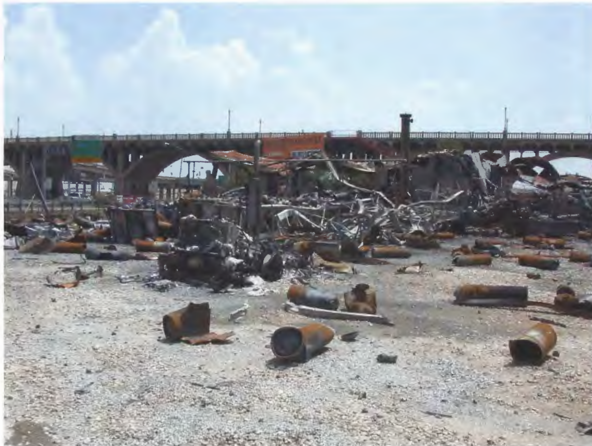
Figure 10. Dallas accident damage to Southwest facility and vehicles. (Accident trailer and cylinders in foreground.)
