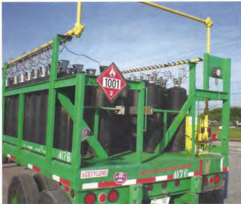
Figure 2—Rear view of typical acetylene trailer
