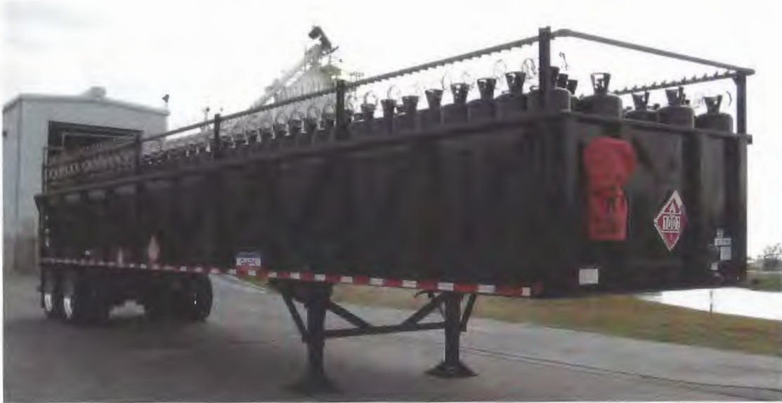
Figure 1—Typical acetylene trailer
