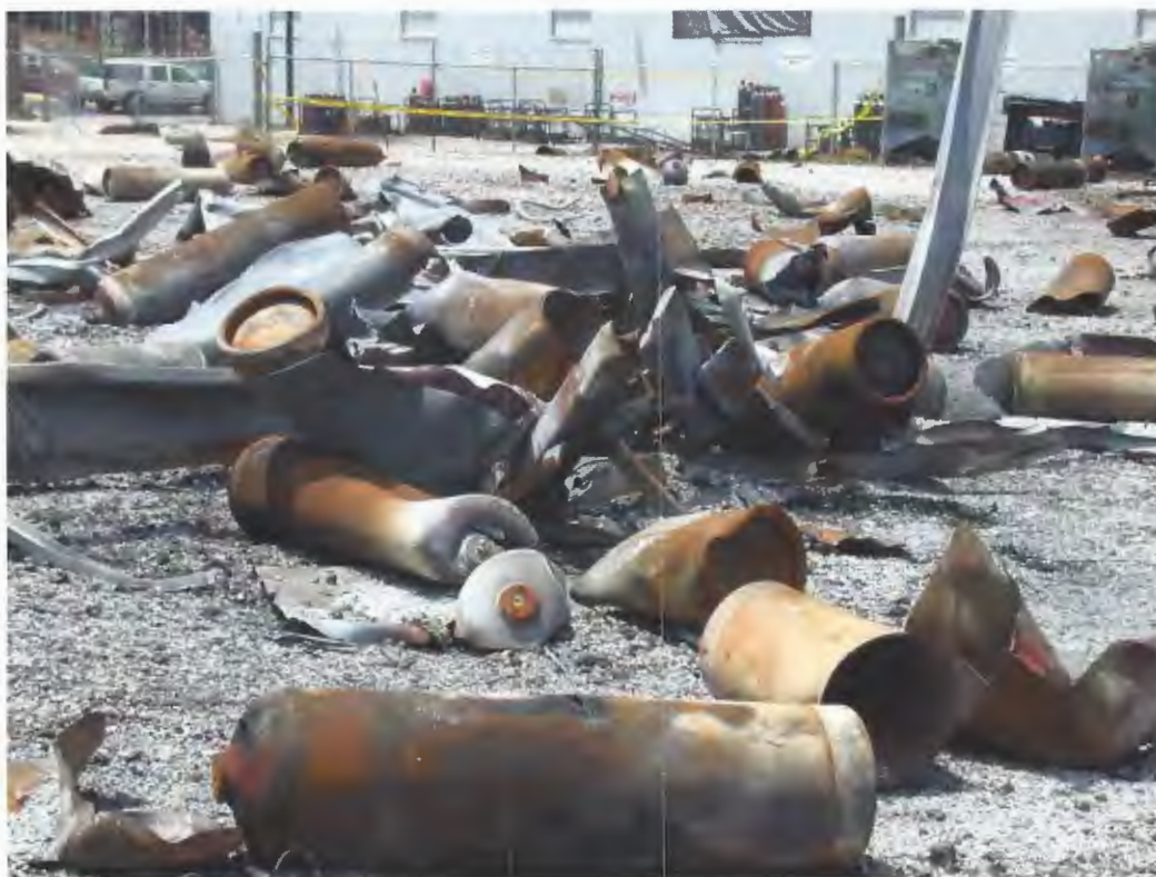
Figure 12. Dallas cylinder damage.
