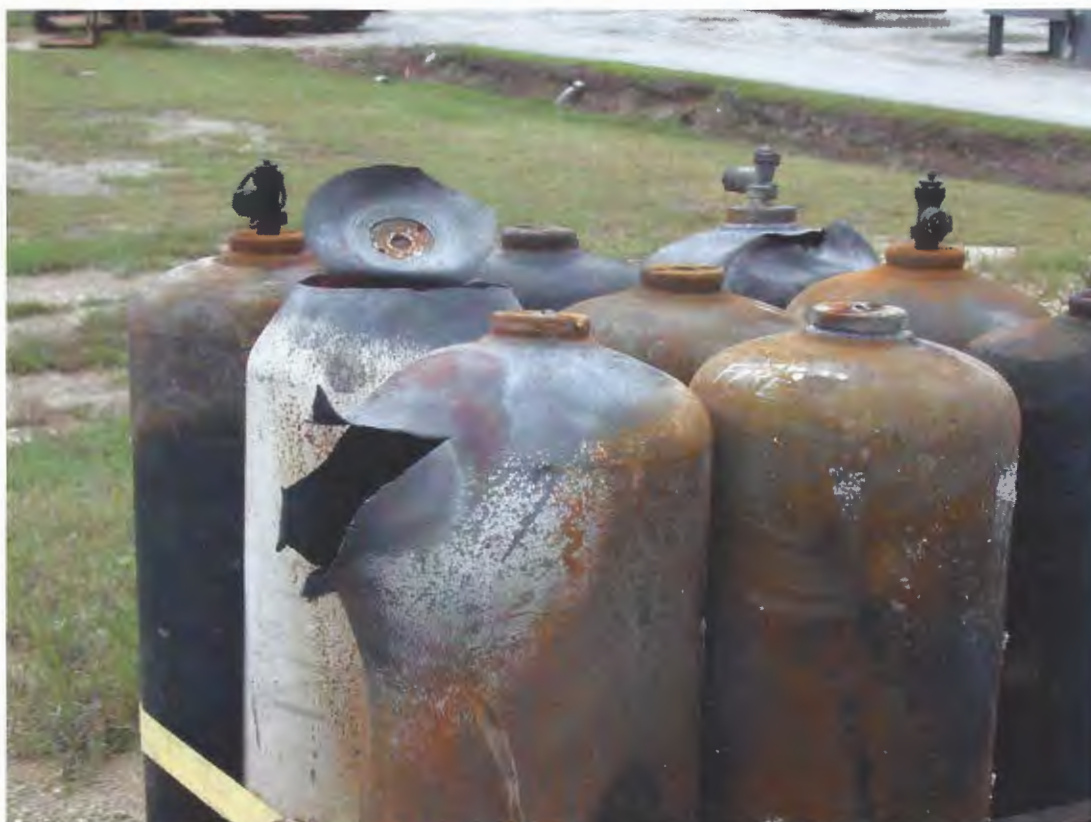
Figure 5. East New Orleans cylinder showing burst near head.
