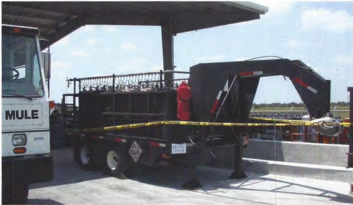
Figure 1. The Woodlands trailer (a small mobile acetylene trailer).
