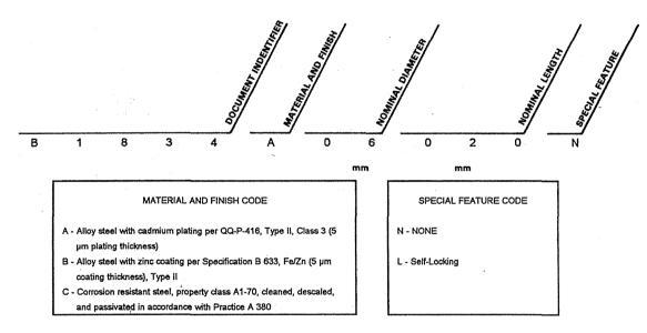
Example: B1834A06020N indicates a Screw Cap, Hexagon Socket Button Head, SI, made of Cadmium Plated Alloy Steel, 6 mm in diameter, 20 mm in length, and no special feature
