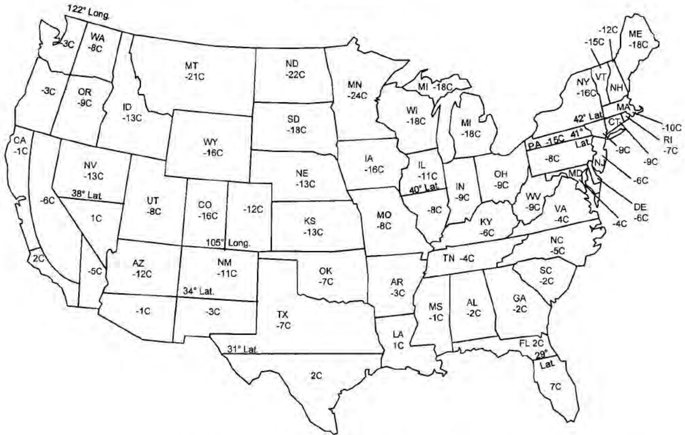
FIG. X5.6 March—10th Percentile Minimum Ambient Air Temperatures
