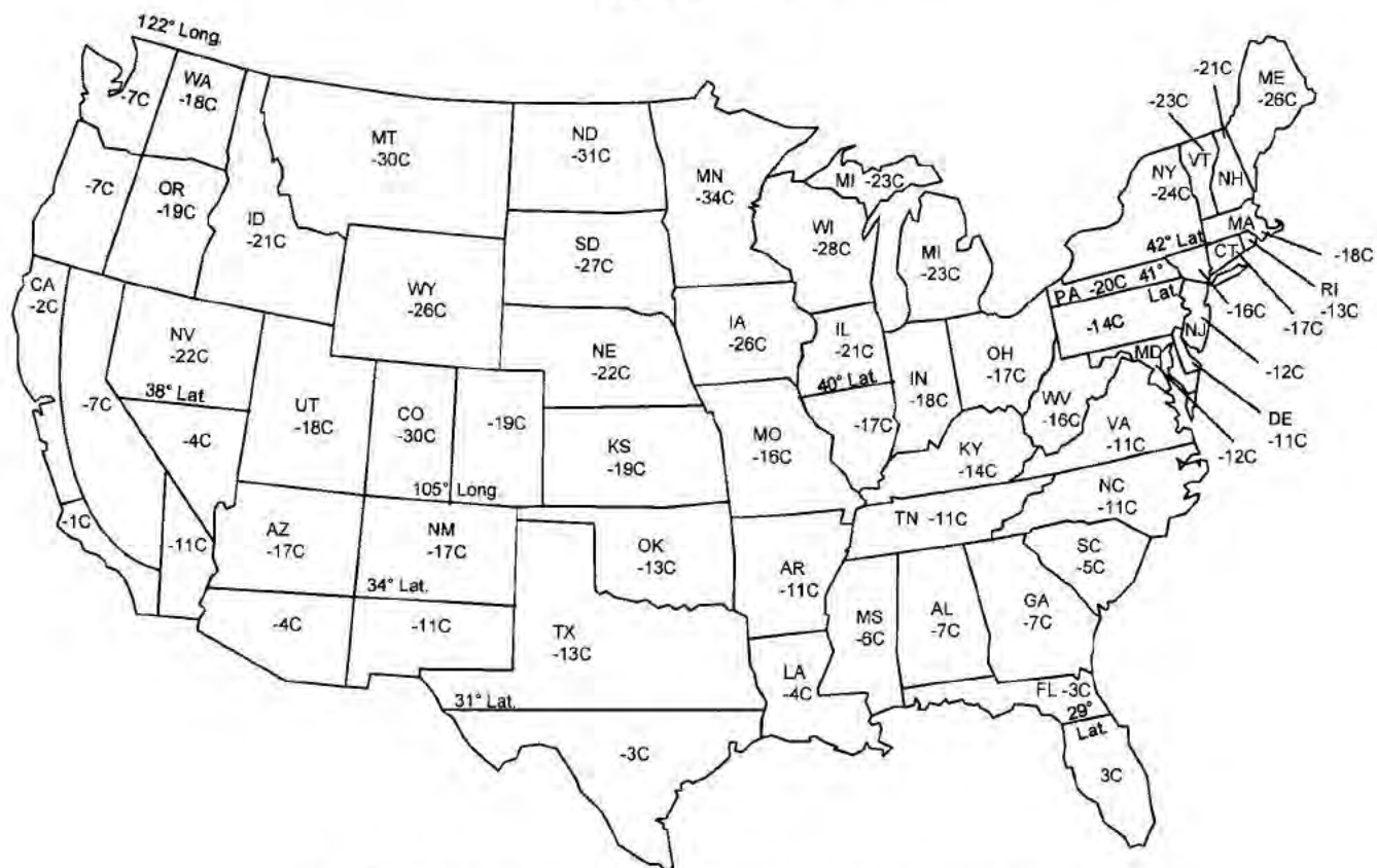
FIG. X5.4 January—10th Percentile Minimum Ambient Air Temperatures
