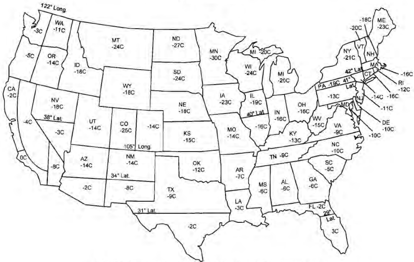
FIG. X5.3 December—10th Percentile Minimum Ambient Air Temperatures
