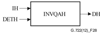
**Figure 28 – Inverse quantization of the difference signal in the higher sub-band**
