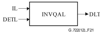
**Figure 21 – Inverse quantization of the difference signal in the lower sub-band**
