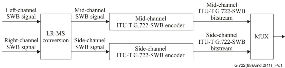
**Figure V.1 – Encoder block diagram of MS stereo using ITU-T G.722-SWB**
