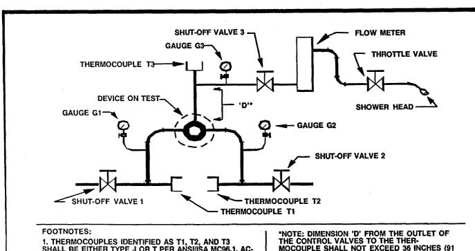
1. THERMOCOUPLES IDENTIFIED AS T1, T2, AND T3 SHALL BE EITHER TYPE J OR T PER ANSI/ISA MC96.1. AC-CURACY AT THE MEASURING DEVICE SHAL BE TO PLUS OR MINUS 1 DEGREE FAHRENHEIT (0.6 DEGREE C.)
