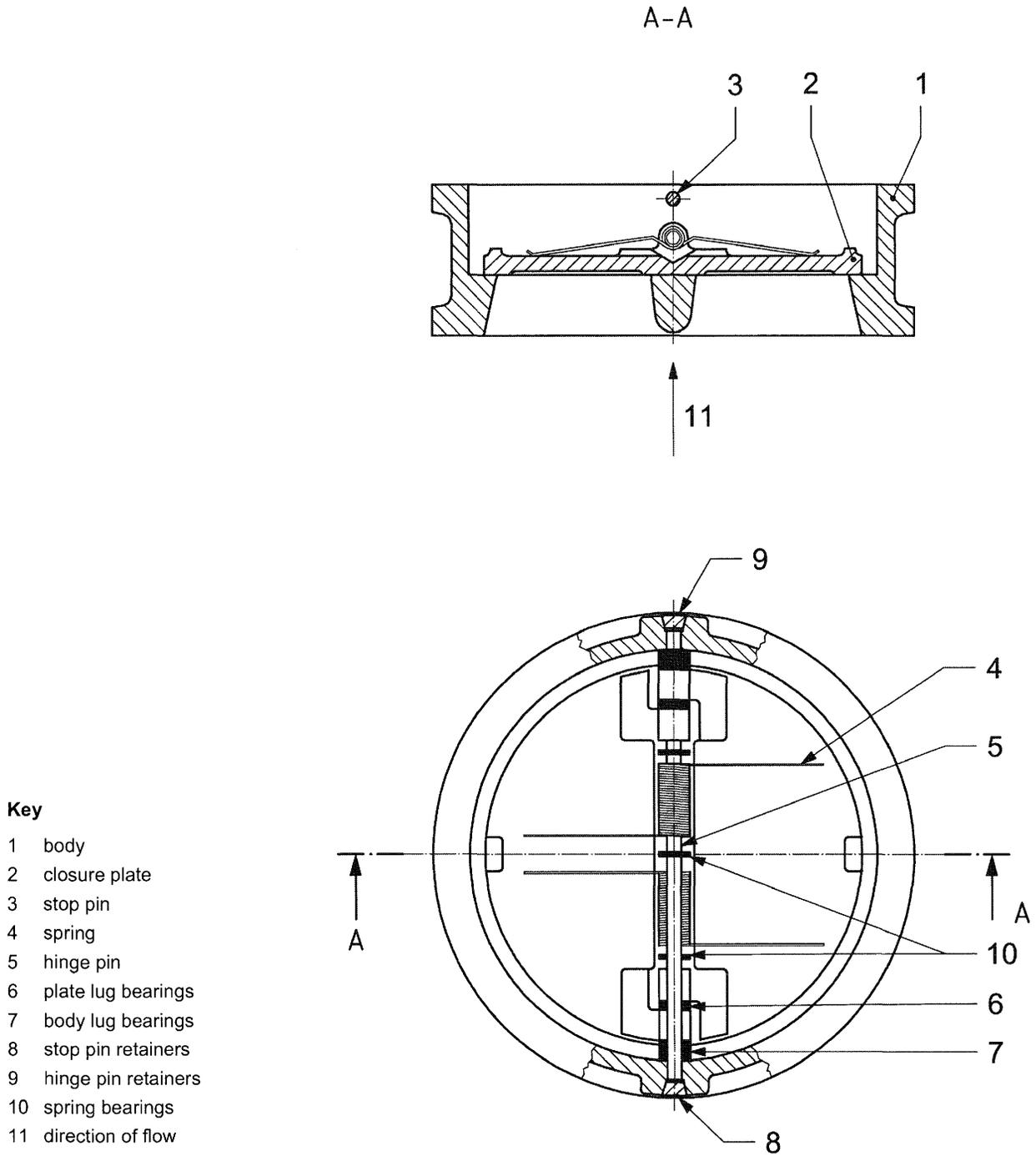
**Figure 10 — Typical dual-plate wafer-type check valve, long pattern**
