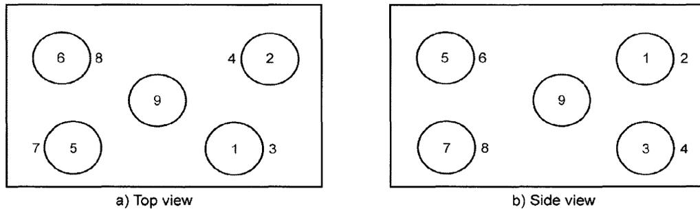
**Figure H.1—Thermocouple location—Rectangular furnace (working zone)**
