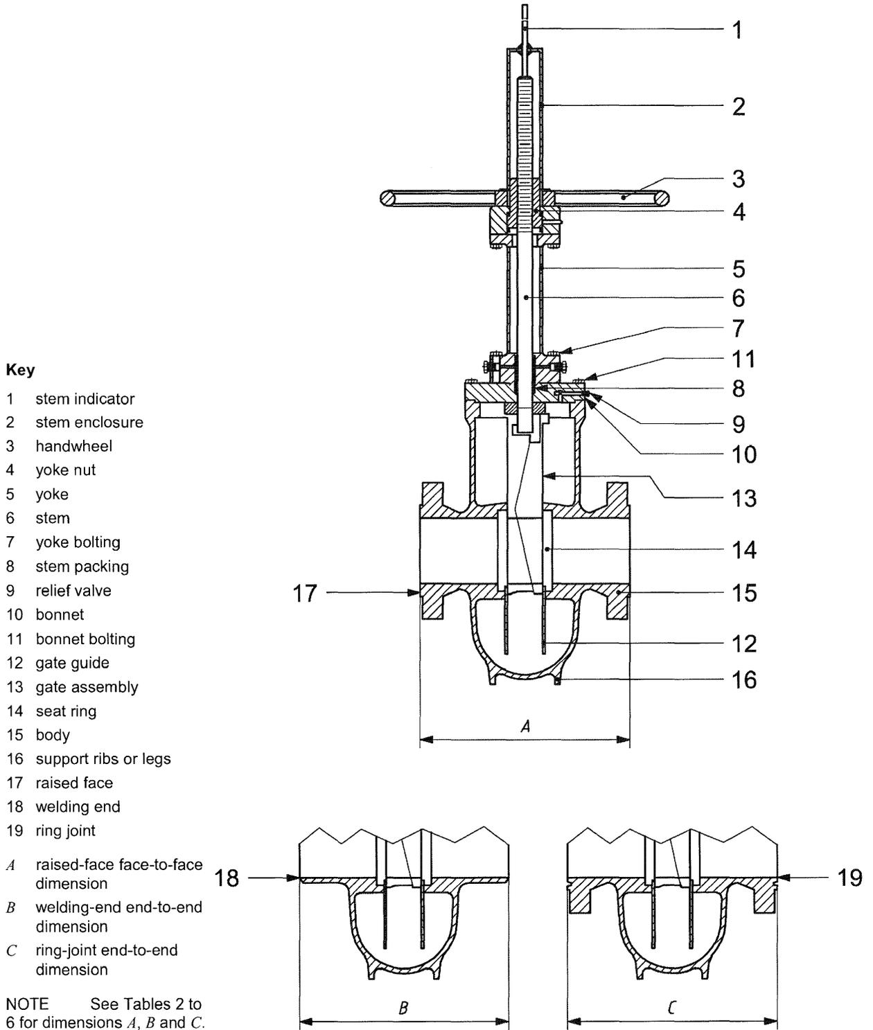
**Figure 1 — Expanding-gate/rising-stem gate valve**
