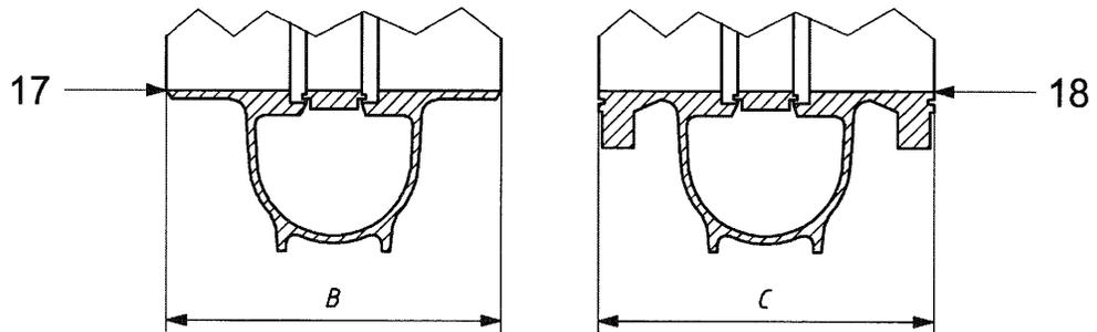
**Figure 2 — Slab-gate/through-conduit rising-stem gate valve**
