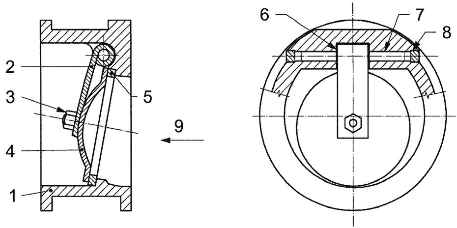
**Figure 9 — Single-plate wafer-type check valve, long pattern**
