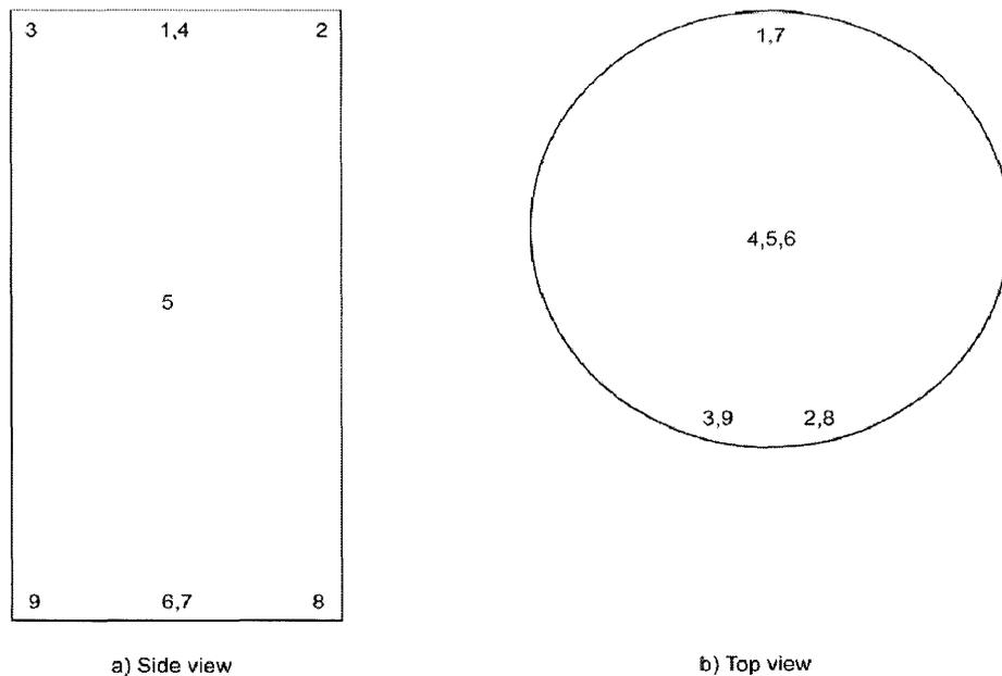
**Figure H.2—Thermocouple locations—Cylindrical furnace (working zone)**
