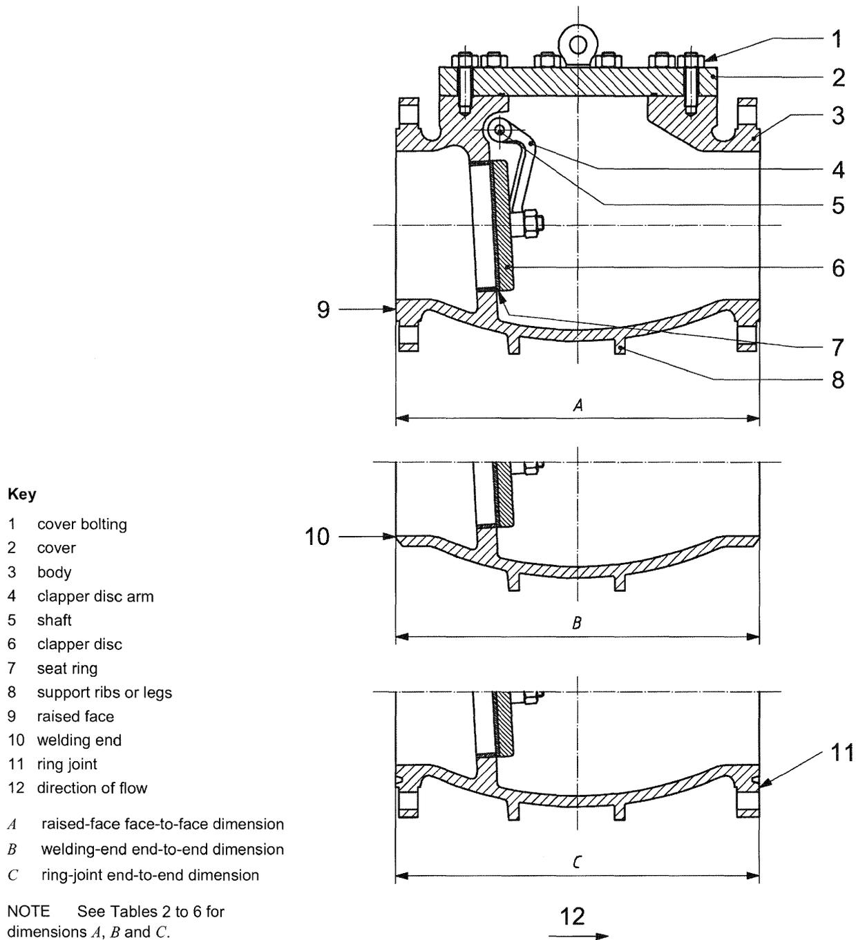
Figure 7 — Reduced-opening swing check valve
