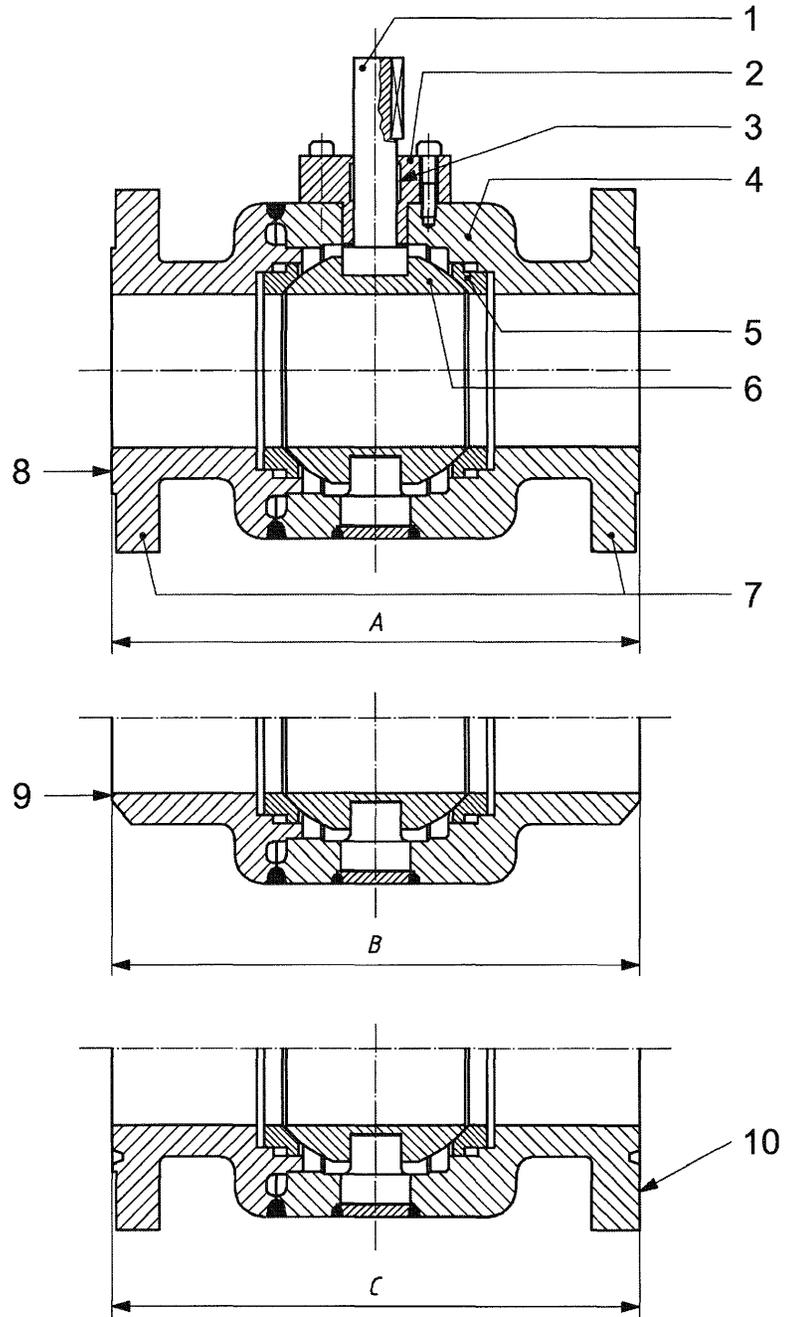
Figure 6 — Welded-body ball valve
