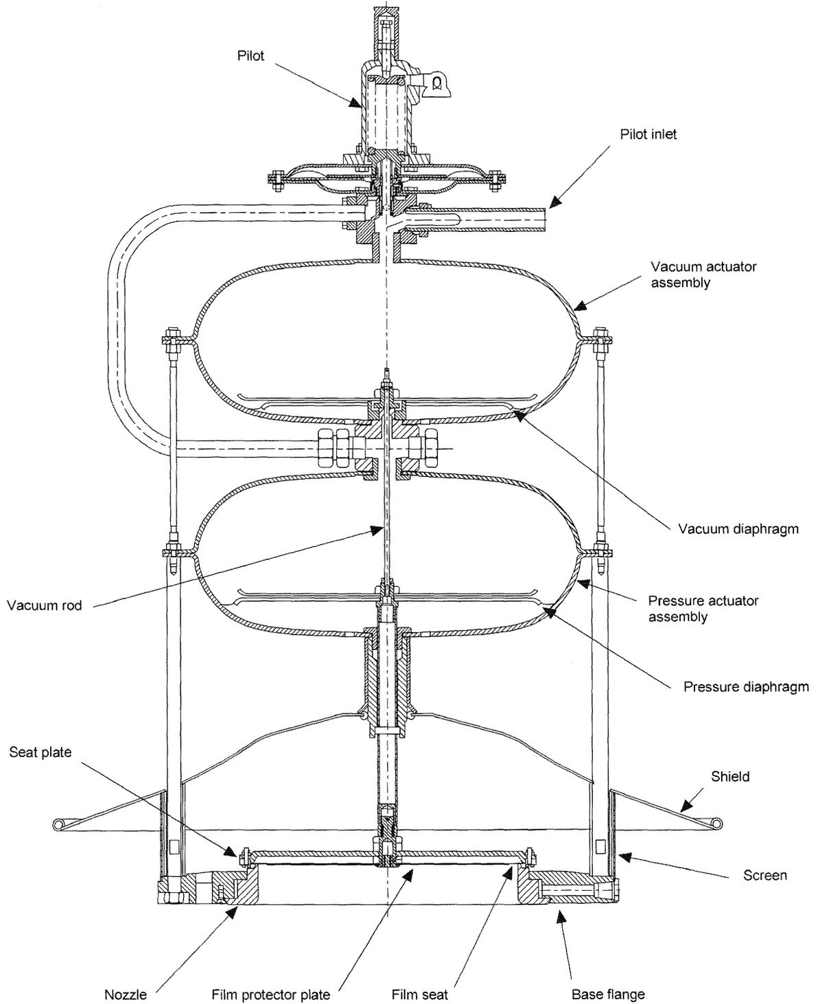
Figure C-7—Pilot-Operated Pressure/Vacuum (Double Diaphragm)
