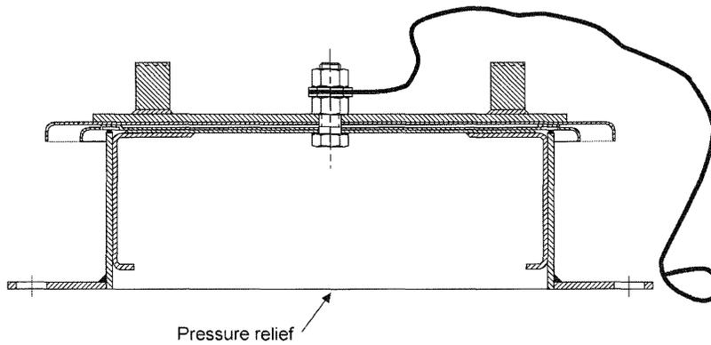
Figure C-3—Large Weight-Loaded Emergency Vent
