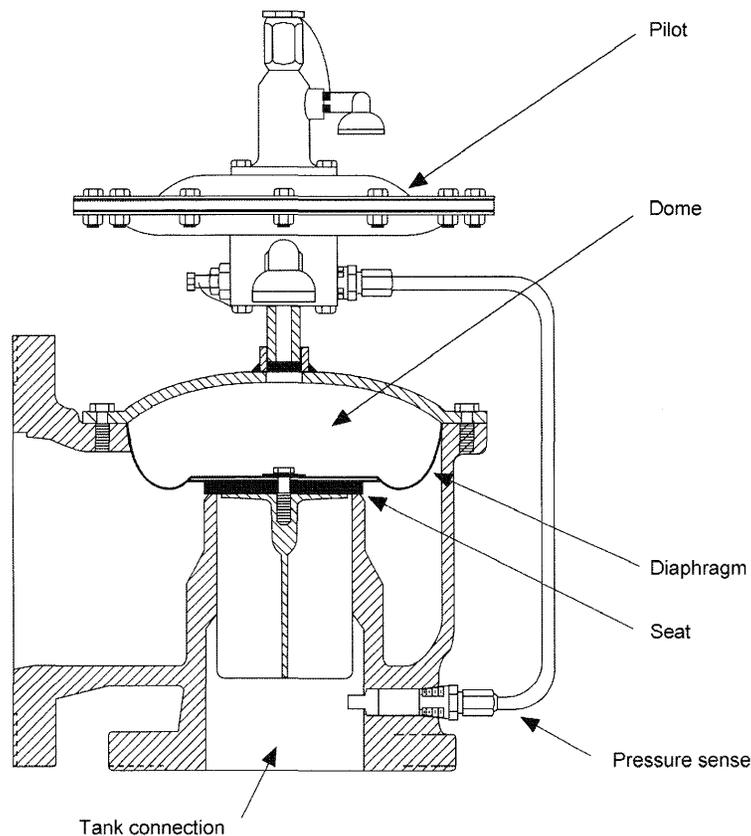
Figure C-6—Pilot-Operated Pressure Vent (Single Diaphragm)
