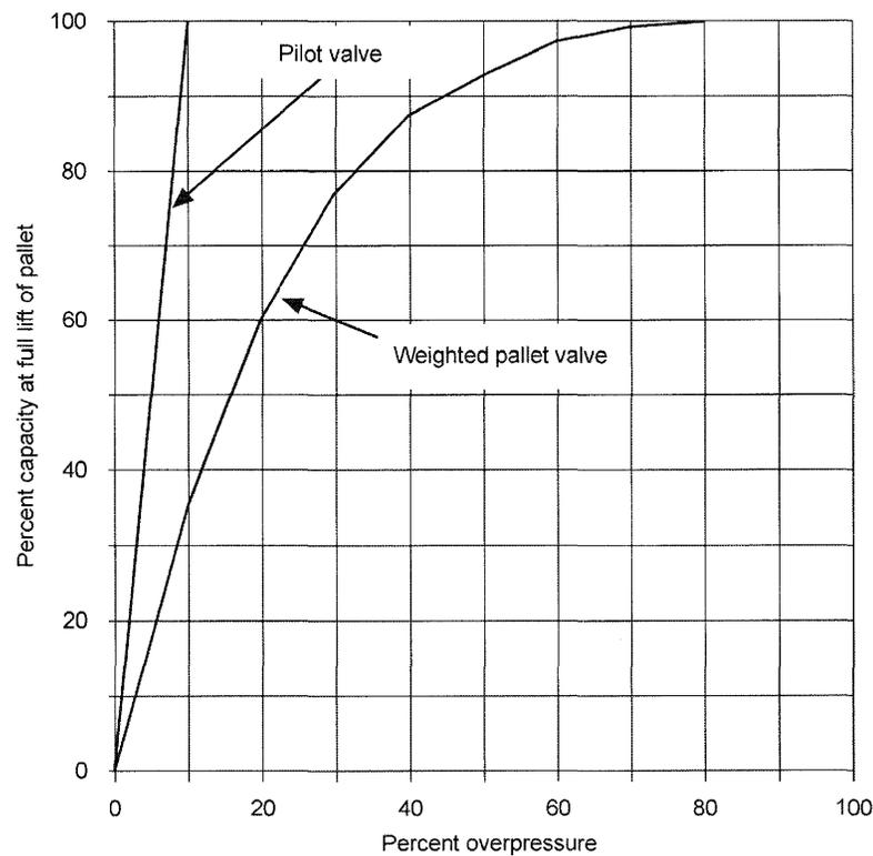
Figure C-5—Capacity/Overpressure Characteristic of Vent
