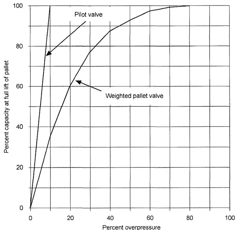
Figure C-5—Capacity/Overpressure Characteristic of Vent
