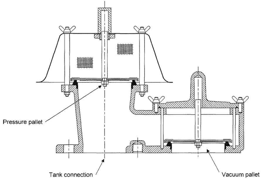
Figure C-2—Side-by-Side Pressure/Vacuum Vent
