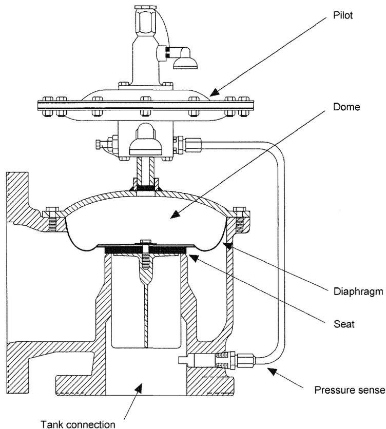
Figure C-6—Pilot-Operated Pressure Vent (Single Diaphragm)
