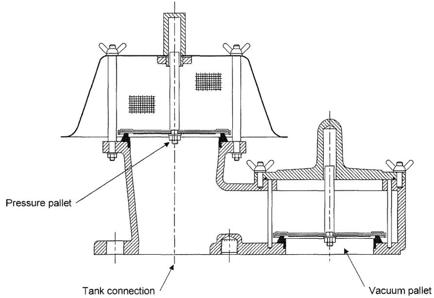
Figure C-2—Side-by-Side Pressure/Vacuum Vent
