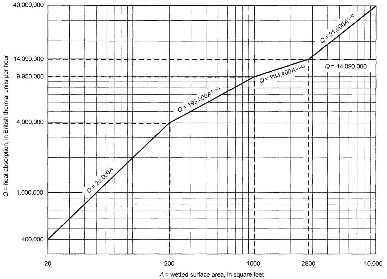
Note: Above 2,800 square feet of wetted surface area, the total heat absorption is considered to remain constant for nonrefrigerated tanks below 1 pound per square inch gauge. For nonrefrigerated tanks above 1 pound per square inch gauge and for all refrigerated tanks, the total heat absorption continues to increase with wetted surface area. This is the reason why the curve splits above 2,800 square feet.
