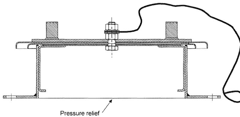
Figure C-3—Large Weight-Loaded Emergency Vent
