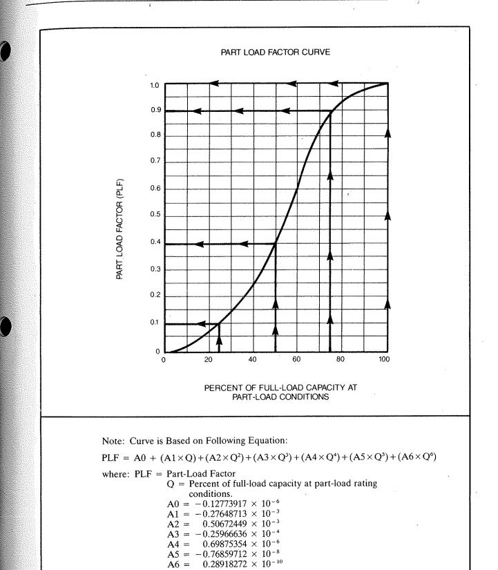
Figure B1. Part-Load Factor Example
