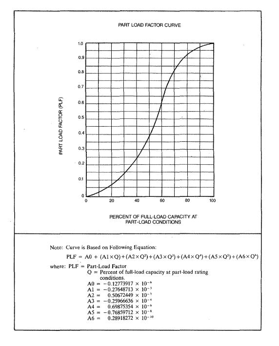
Figure 1. Part-Load Factor Curve
