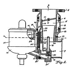
From the fuel reservoir 15, through the passage 17, gasoline is fed through the orifice 21 into the main jet within the Venturi tube, and also is fed through the orifice 27 into the auxiliary reservoir 25, and thence into the supplemental jet 33. The auxiliary reservoir 25 is open to the atmosphere through the restricted opening 31, and it is also open to the chamber 28, in which are openings 29 and 30 into the Venturi tube
