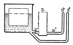
B<sup>4</sup> is the suction jet; D<sup>2</sup>, the supplemental jet. Air-leg D, of the auxiliary well D D1 D2. is indicated by the dotted lines. This was for the purpose of showing, first, that the Baverey principle could be used without the presence of the air-leg D; and, second, that its presence was merely incidental, therefore not to be counted in determining infringement. If a
