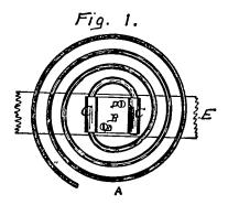
Obviously the inturned end of the metal plate B in Crandall's patent, embracing the bottom coil of the supported spring, completely
