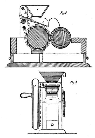
The essential features of this patent are a toothed cylinder, the spaces between the teeth being narrower than the thickness of a raisin seed, a single rubber roll adjacent to the toothed cylinder, by means of which the raisins are impaled upon the teeth and the seeds excluded therefrom, suitable feeding devices, and means for stripping from the toothed cylinder the seeds and pulp of the fruit.
