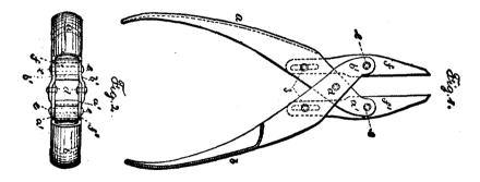
Patent No. 427,497: "(2) The combination, with the lever handles having crosspleces riveted together, of the jaws, A, B, and the rivets or screws connecting the same to the lever handles; the jaw, B, having an arm, F, formed with or connected to it, and extending along the back of the jaw, and a punch, G, passing transversely through the parallel moving jaws, and a counter die in the end of the arm, against which the punch acts, substantially as set forth."
