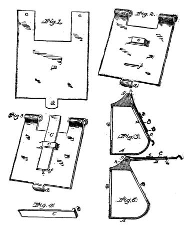
holding the lower end of the spring from lateral displacement. Other means are provided for this purpose in the Kinzer lid, consisting of the long, cast ribs i, i, which laterally confine the spring from the loop, H, to the lower end of said spring."
