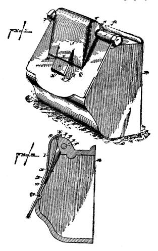
place." The difference in detail consists in the use of a bulged or hooded lid, the form of which was old in cast iron but new in being made from pressed steel, and having a slot at its lower end, through which the spring entered. Apart from sheltering the upper end of the spring beneath it, the hood performed the same functional duty of a bearing point of the spring as the raised loop of the former patent. The seating of the spring still remained on the outside of the
