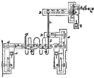
"(3) The roll train, D, arranged with its rolls in, or approximately in, line with the last or delivery rolls of train, B, and the first or receiving rolls of train, C, C', in combination with said rolls, B, and C, C', and with the trough, b, or other suitable means, as described, whereby provision is made for turning the bar or billet intermediate between said trains, B and D, substantially as set forth.
