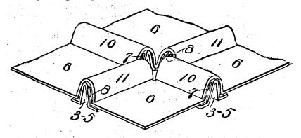
The figures 3-5 show the angle strip running from the ridge to the eaves; 6 shows the sheet with its upright flange, 7, lying against one side of the angle strip; 6-10 shows the next adjacent sheet, with its inverted U-shaped flange, 10, overlapping flange 7 and the angle strip,—making altogether the upright joint extending from the ridge to the eaves, constituting the combination under the first claim of the patent. The figures 3-5, in combination with 11 and
