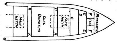
H, H, and K, K, were beams running across the vessel, each 2 feet wide. They were on the same level with the other between-deck beams. A stringer of iron, G, G, 1 foot 9 inches wide in parts, and 2 feet wide in other parts, v.50r.no.2—15
