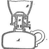
the lamp, B the wick-tube, E the chimney, & the chimney-rest, and F the cone or deflector, provided around its upper edge with peripheral springs, or having the edge cut into radial slits, h, the function of which is to press against the glass of the chimney and hold it in place.]<sup>2</sup>
