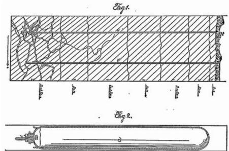
"What I claim as my invention, and desire to secure by letters patent, is: The above described method of increasing the productiveness of oil wells by causing an explosion of gunpowder, or its equivalent, substantially as above described.
