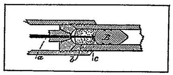
In the Prussian needle-gun, cited as reference, of which an illustration istaken from patent to Polnice, No. 11,835, October, 1854, the charge is fired at the same point, but by different devices. A needle a passes through the charge b, and explodes a fulminate c placed against the rear end of the bullet B.
