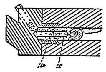
The applicant's invention will be readily understood from the subjoinedcut taken from the patent subsequently issued to him in accordance with this decision, No. 15,292, July 8th, 1856; a represents the priming-tube for conducting the flash of the cap to the forward part of the charge c, and sofiring the same at that point and just behind the ball B.
