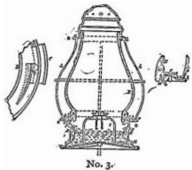
No. 3 is an engraving of the Waters lantern, in which the guard-rods are attached at their lower ends to a ring connected with the band which sustains the globe, by lips extending over the ring on one side and a spring-catch on the opposite side of the globe.
