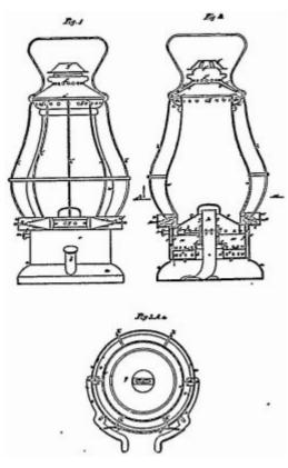
ring or jacket was intended to protect the air in the flame chamber from disturbing outside currents, and secure a steady flame, while the function of the deflector, q, was to deflect or concentrate all the air that entered the flame chamber to the base of the flame within the boss. In this combination, the globe of the lantern acts as a chimney to the burner, and at the same time protects the flame from external air.
