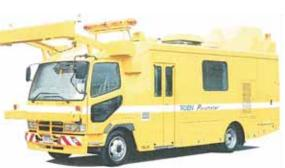
Fig. 6.05N Road Surface Survey Vehicle
