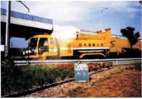
Fig. 6.05G Watering Machine for Horticulture
