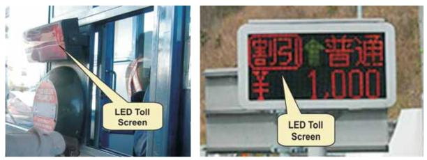
Fig. 1.03 LED Display (showing Toll Rate)
