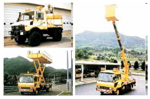
Fig. 6.05C Portable Lift on Truck
