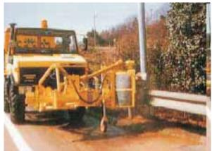
Fig. 6.05F Self Propelled Cleaning Machine for Drainage
