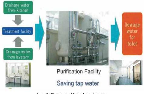
Fig. 3.08 Typical Recycling Process (Source : Japan Documents)
