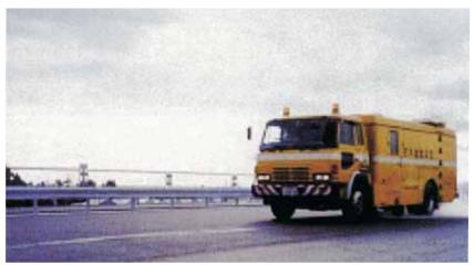
Fig. 6.05P Skid Test Vehicle (for Skid Resistance)
