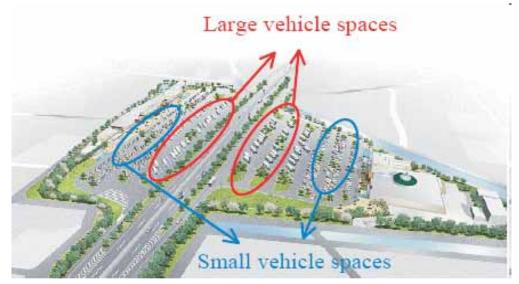
Fig. 3.27 Parking Layout for Segregation Between Large and Small Vehicles (Source : Japan Documents)
