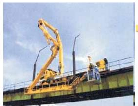
Fig. 6.05M Bridge Inspection Vehicle
