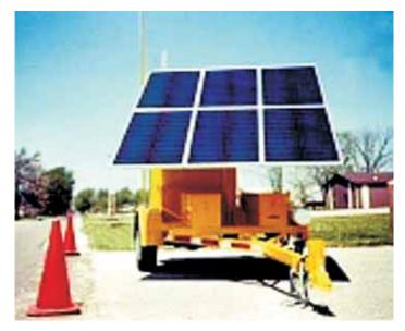
Fig. 2.09 Portable Highway Advisory Radio Station
