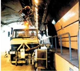
Fig. 6.05I Tunnel Wall Cleaning Machine
