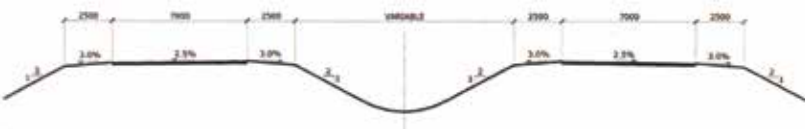
Fig. 10.2. Cross Section of a four lane rural highway with depressed median without lined saucer drain
