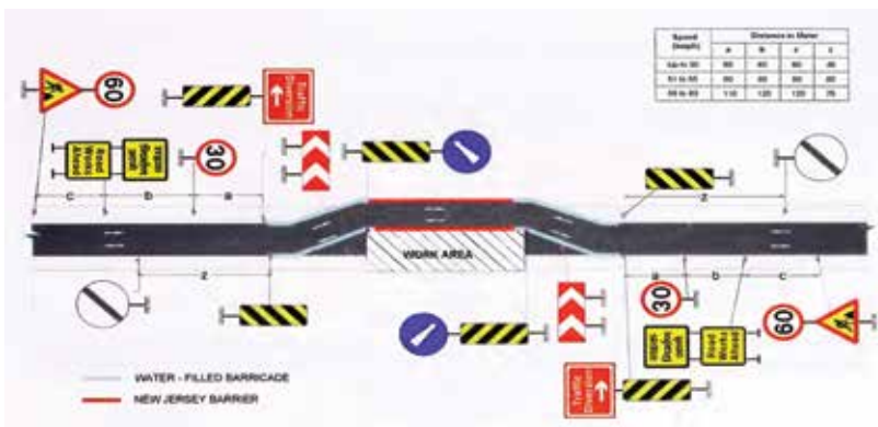
Fig. 7.18 Upgrading of 1 L / Intermediate Lane to Two Lane with Shoulders
