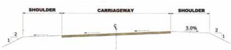
Fig. 10.1. Typical One-way Camber in Super Elevated Sections
