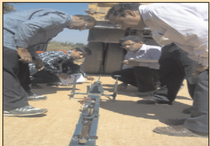
Figure 14 Quality testing after construction by core extraction and Benkel Beam Deflection test
