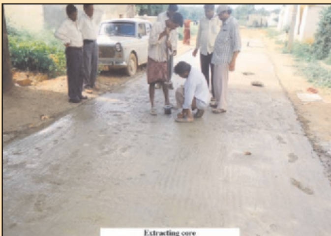
Figure 14 Quality testing after construction by core extraction and Benkel Beam Deflection test
