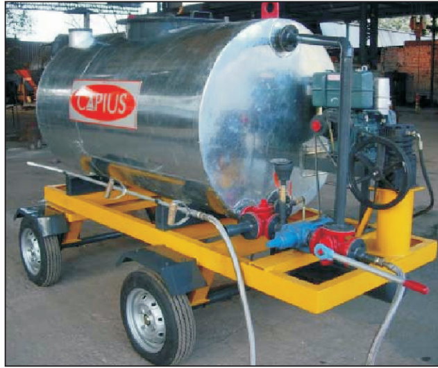
Fig. 9.4 Bitumen Sprayer Mounted on Pneumatic Tyres
