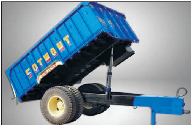
Fig. 11.8 Single Axle Trolley Fitted with Hydraulic Tipping Arrangement
