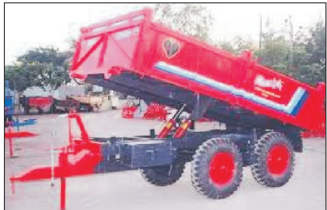
Fig. 11.9 Double Axle Trolley Fitted with Hydraulic Tipping Arrangement
