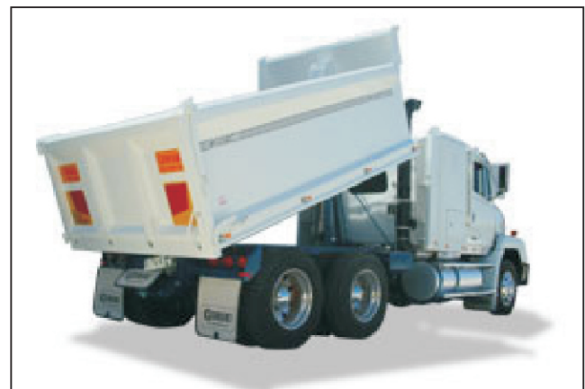
Fig. 11.2 Tipping Truck on Tandem Axle
