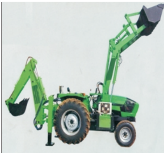
Fig. 4.3 Tractor fitted with Loader and Back Hoe Attachment
