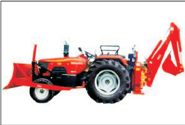
Fig. 4.5 Tractor fitted with Dozing and Backhoe Attachment
