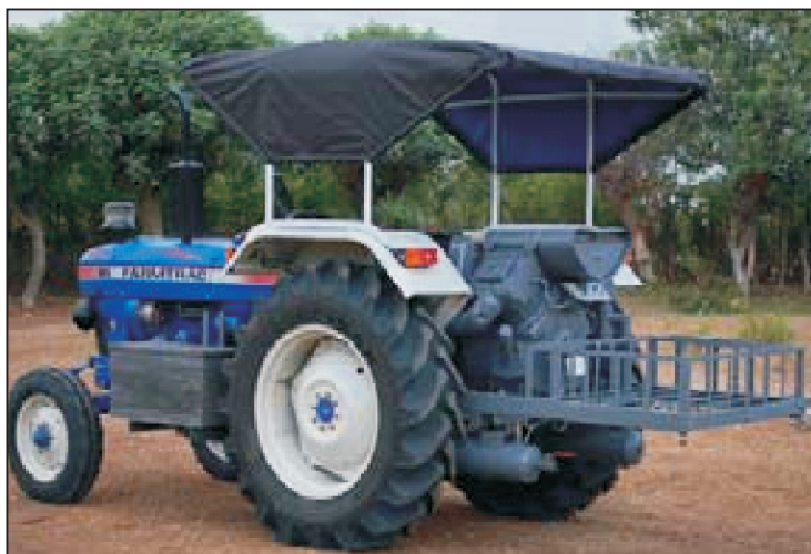
Fig. 14.1 Air Compressor Mounted on Tractor
