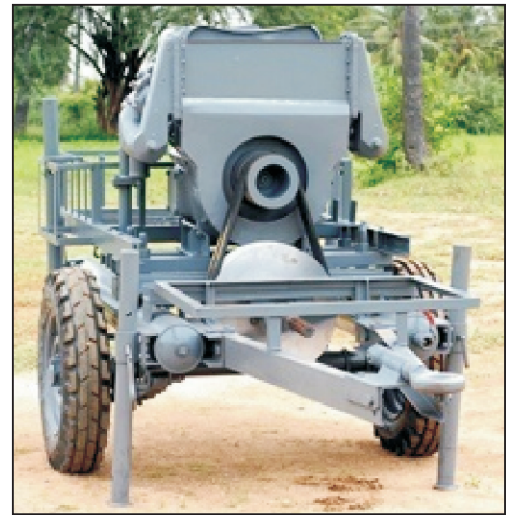
Fig. 11.7 Air Compressor Unit Mounted on Trolley
