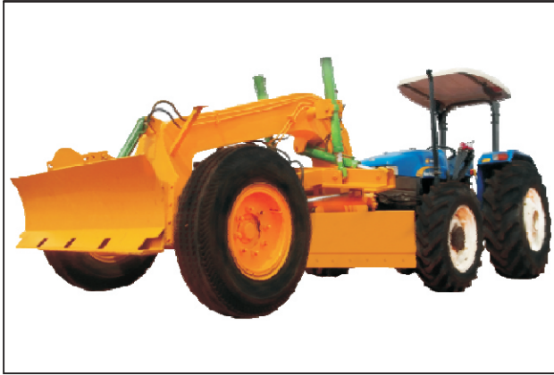
Fig. 4.9 Tractor fitted with Dozing and Grading Attachment
