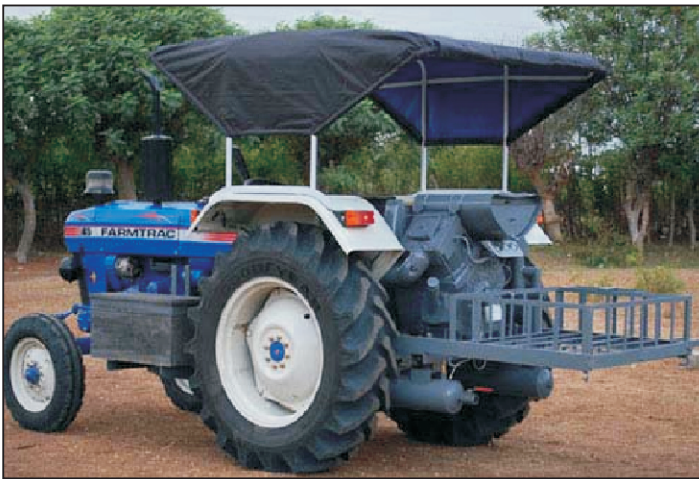
Fig. 11.6 Tractor Fitted with Air Compressor Unit
