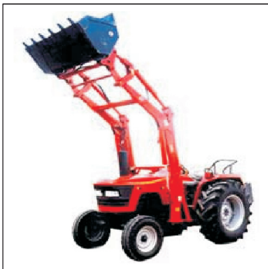
Fig. 4.1 Tractor fitted with Front End Loader Attachment
