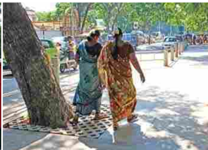
Fig. 72 In Retail/Commercial Areas, MFZ should have trees in Tree-Guards (and not continuous planting strips) – to allow more Space for Pedestrians to walk over, as well as flexibility to disembark from various modes near the Kerb-Edge.
