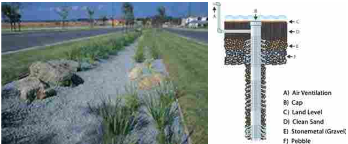
Fig. 47 Percolation/Infiltration Trench in the Median. (Right) A Typical Percolation Pit Detail
