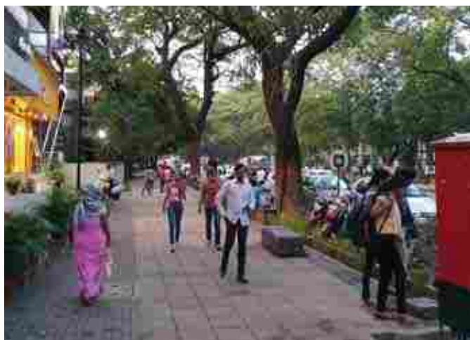
Fig. 71 Continuous Planting Zones within MFZ are suitable where High-Speed Traffic is expected in off-peak hours and Pedestrians need to be contained within the Walking Zone.
