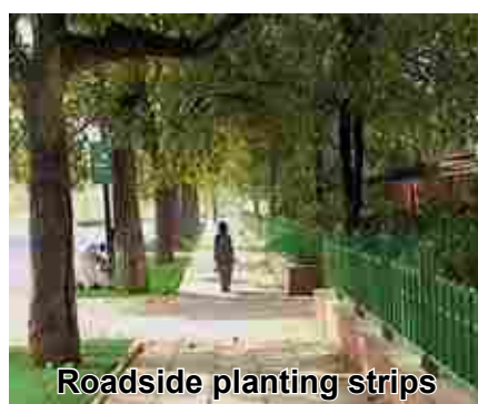
Fig. 60 Areas that could be used for Localized Storm Water Management on Roads: include Roadside Planting Strips (MFZ), Landscaped Medians, Underside of Flyovers and Viaducts, etc.
