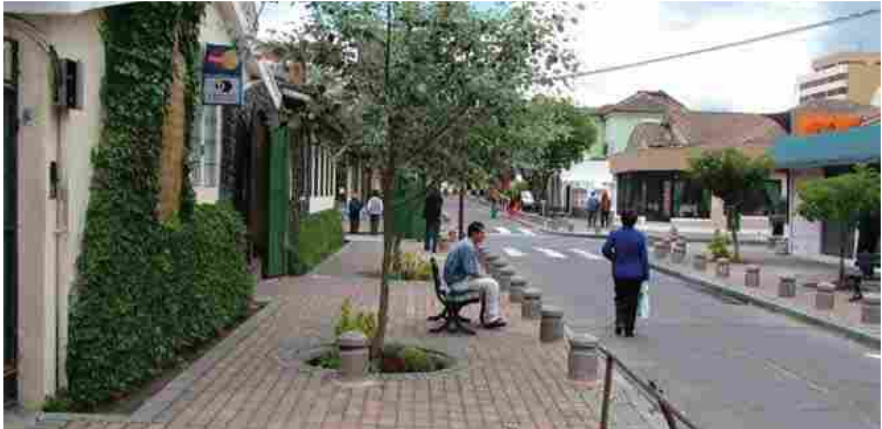
Fig. 33 Use of Bollards to Separate Road from Walking Area.
