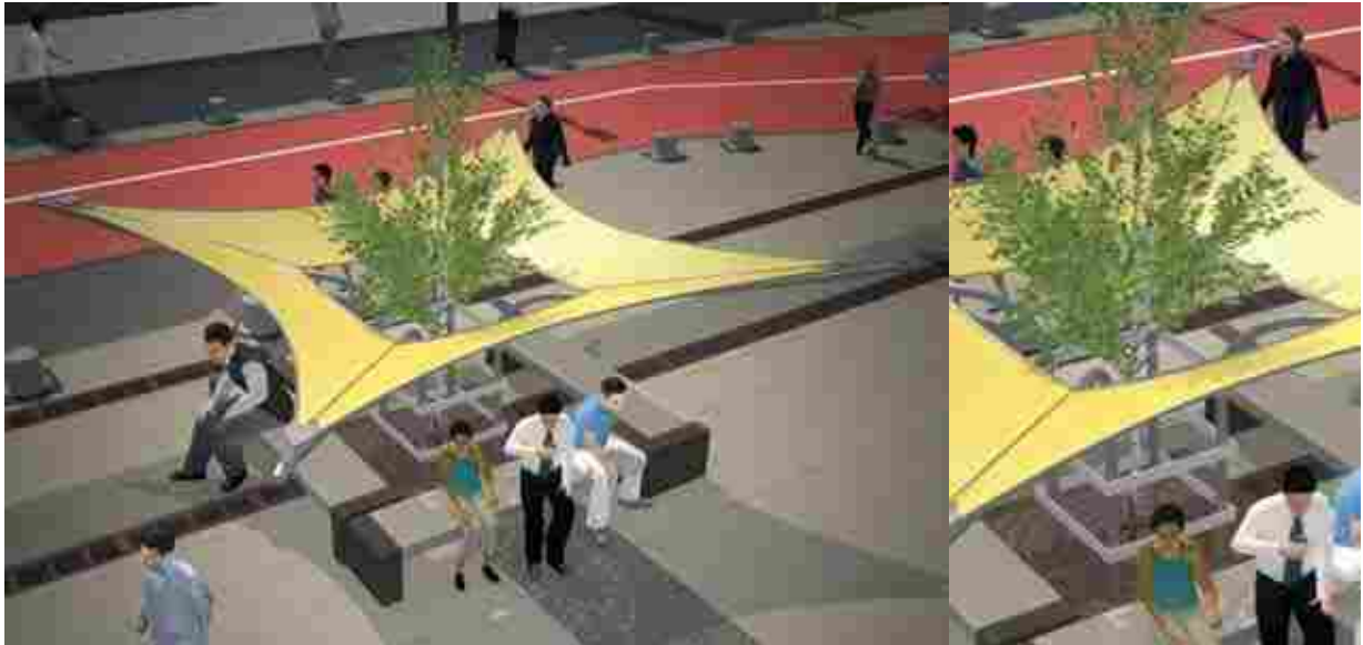
Fig. 106 Tree Guard Detail with Tensile Structure to Protect Trees when they are yet to Mature
