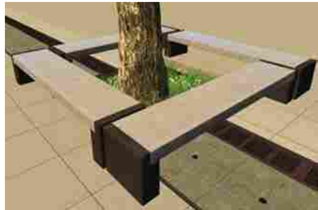
Fig. 96 Tree-pit Detail with Seating
