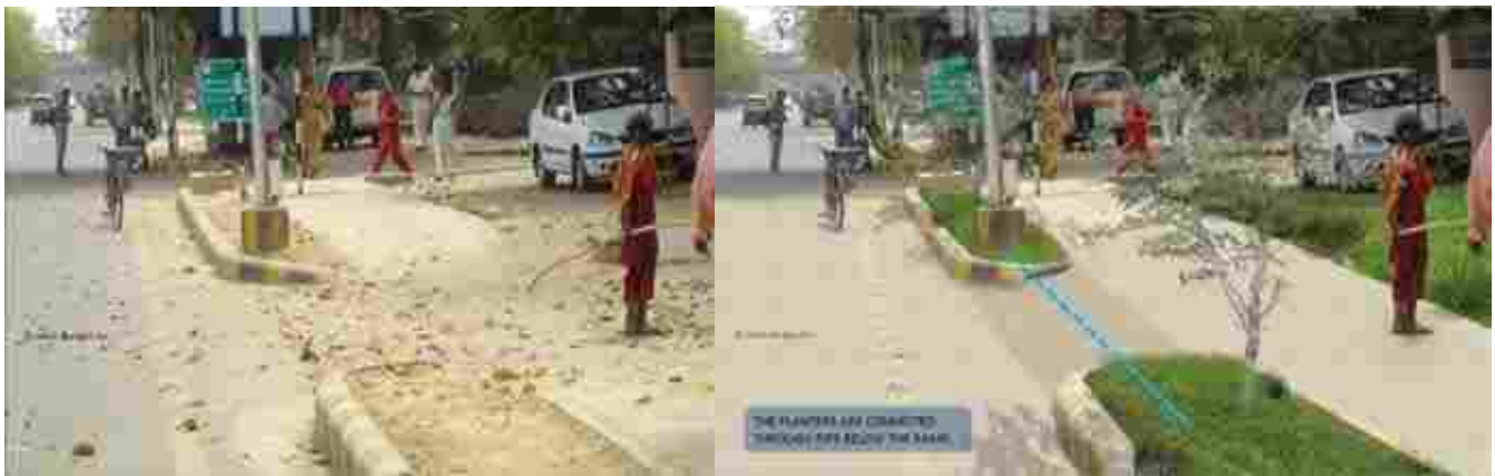
Fig. 56 Existing and Proposed: Green Gutters, although Narrow, can increase Infiltration
