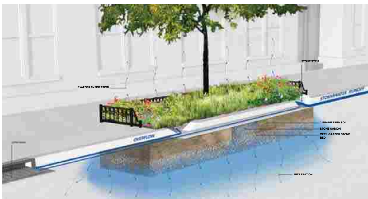
Fig. 88 Bio-planters can be located within the Multi-Functional Zone
