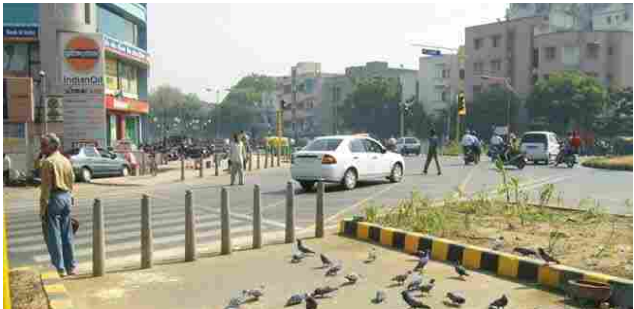
Fig. 34: Use of Bollards to Restrict Intrusion of Vehicles in Pedestrian Refuge Area
