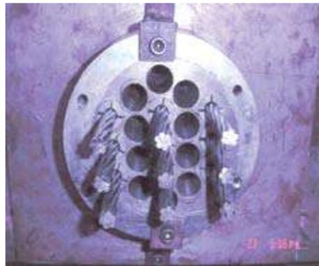
Fig. C13.2.4 (b) Dynamic Load Test : Test Specimen (Partial Tendon) with 9 Strands of 15 mm dia
