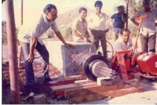
Fig. C13.2.3 Anchor Efficiency Test Using Specially Cast Beam (on 19 Strands of 13 mm Dia - UTS 350 T)
