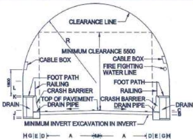
Sketch 1: Section of Two Lane Bi-Directionla Traffic Tunnel
