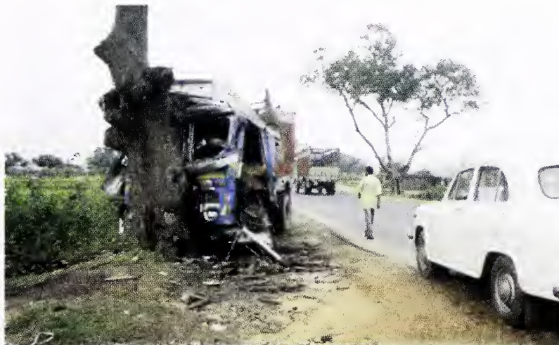
Fig. 5.24 Trees on the Edge of Roadway can be a Cause of Very Severe Accidents
