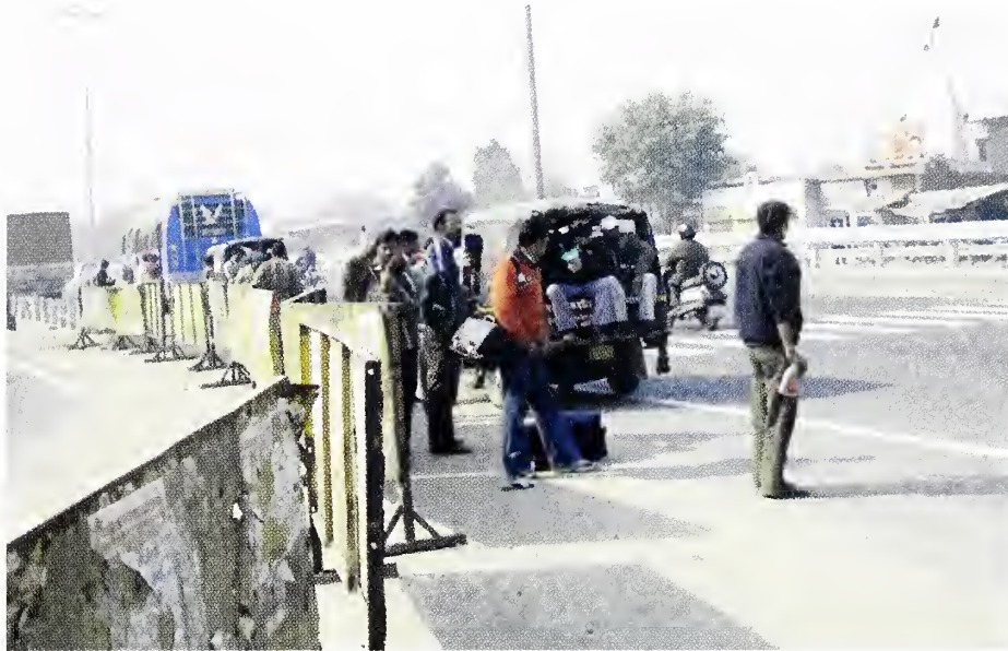
Fig. 6.4 Passengers are Forced to Enter on Main Carriageway in Absence of Bus Bays
