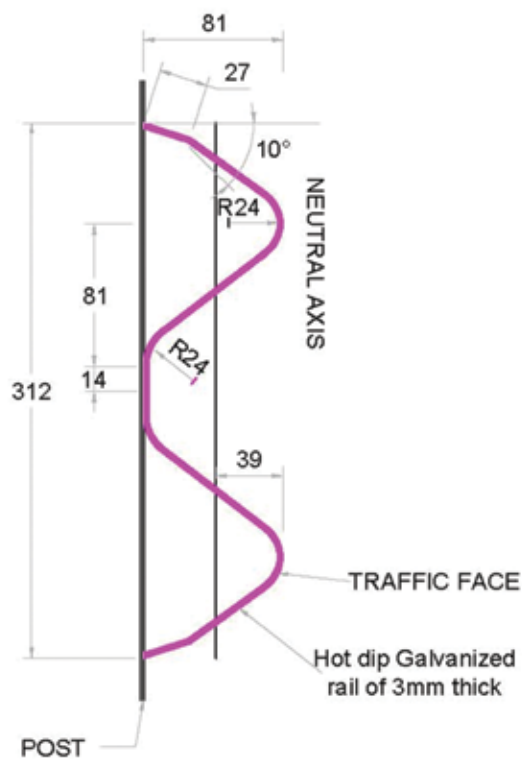
Fig. 9.9 Typical Details of W Beam Structural Elements
