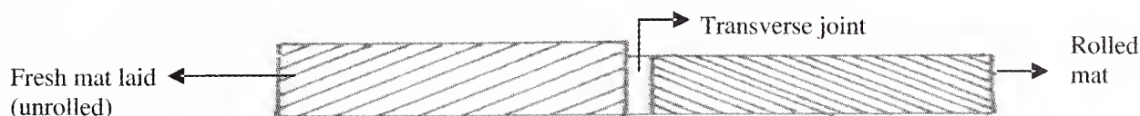
Fig. 25 Formation of Transverse Joint through Perpendicular Process
