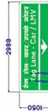
Fig 10.6B: Lane Dedicated Sign (Font Size: Lowercase -120 mm & Uppercase-168 mm)
