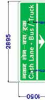
Fig 10.6C: Lane Dedicated Sign (Font Size: Lowercase -120 mm & Uppercase-168 mm)
