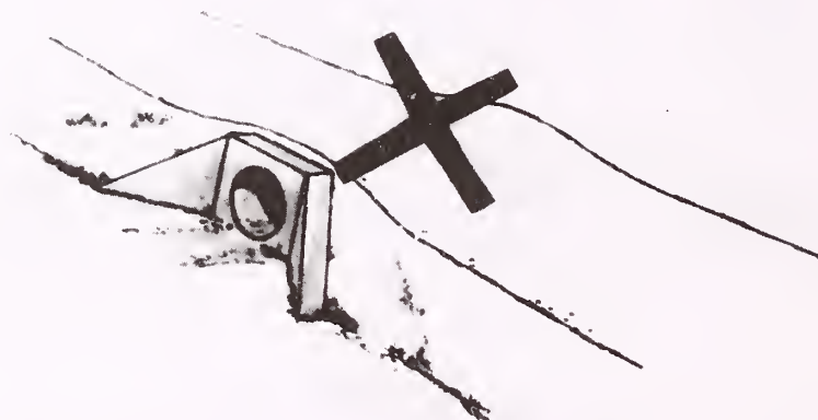
Fig. 4.5 : Avoid Hump at Culvert
