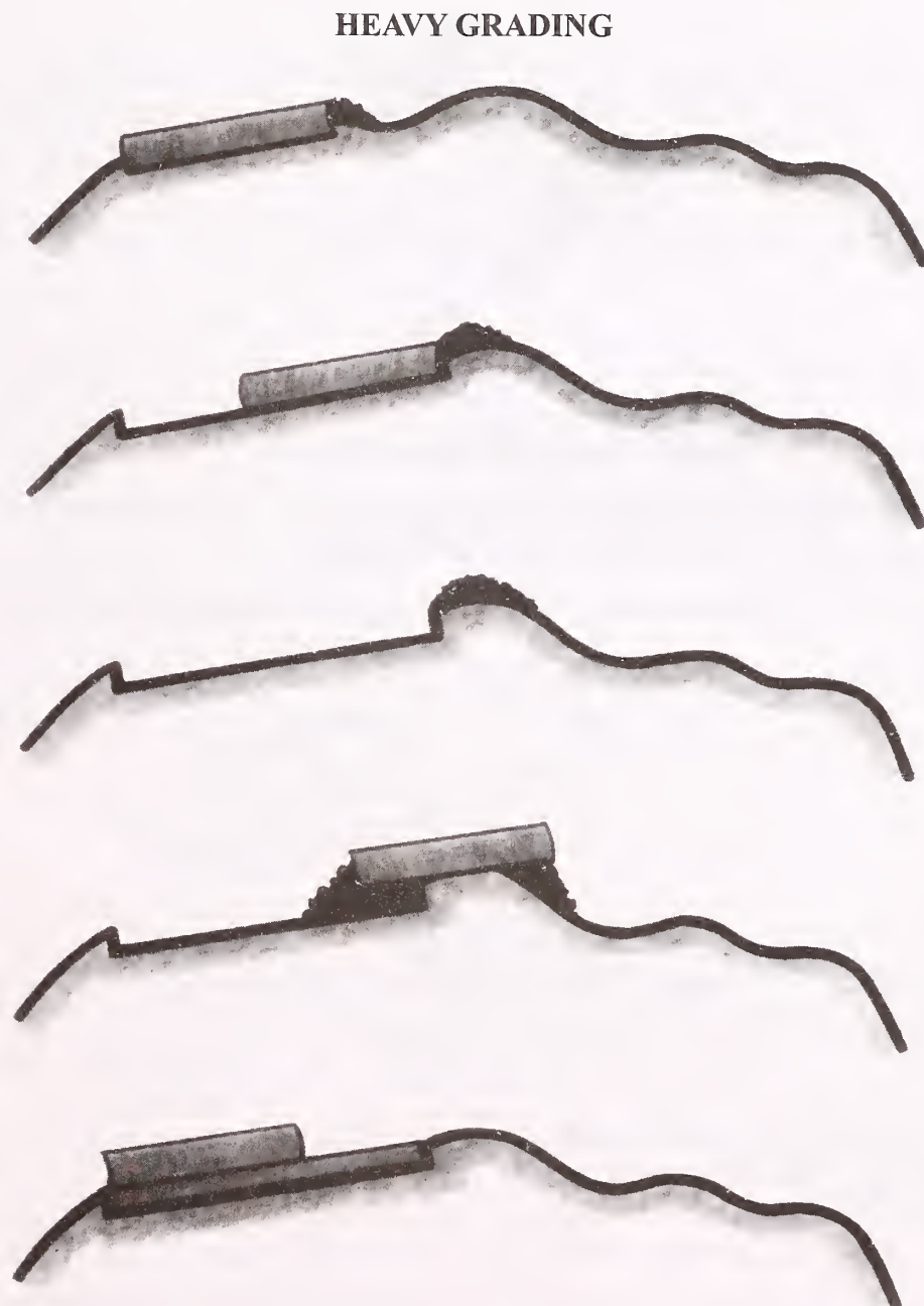
Fig. 4.3 : Light and Heavy Grading
