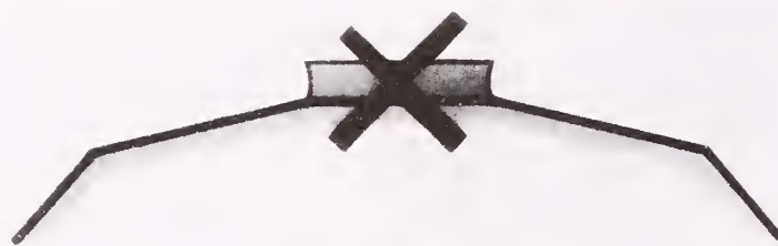
Fig. 4.4 : Avoid Flattening at the Centre (Ref 1)
