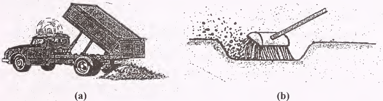
Fig. 4.11:(a) Dump the material on the shoulder adjacent to location of patching work (b) Brush out any loose material or standing water
