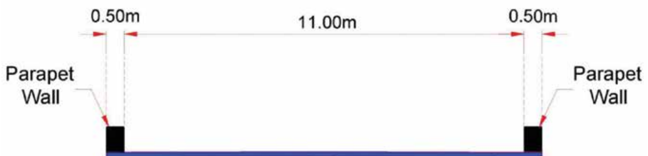
Fig 7.4 Typical cross section of Culvert at deck level for 2-Lane Highway with paved shoulder (Open country - Mountainous terrain)
