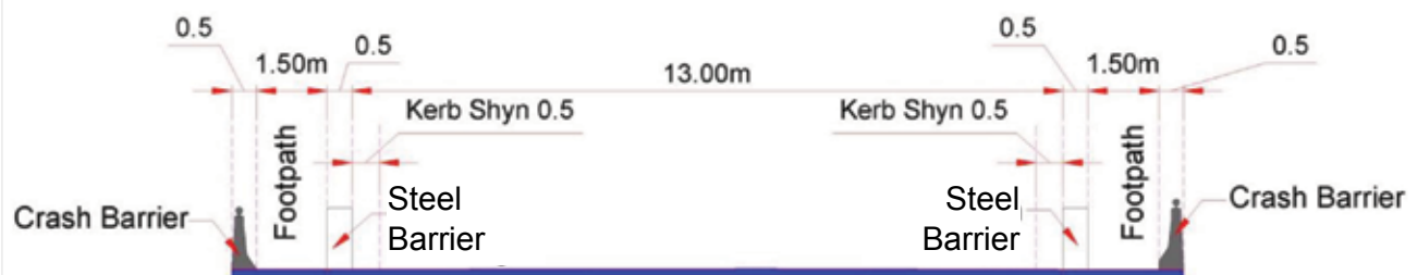
Fig 7.6 Typical cross section of bridge for 2-Lane Highway with paved shoulder and protected footpath (Open country - Plain/rolling terrain)
