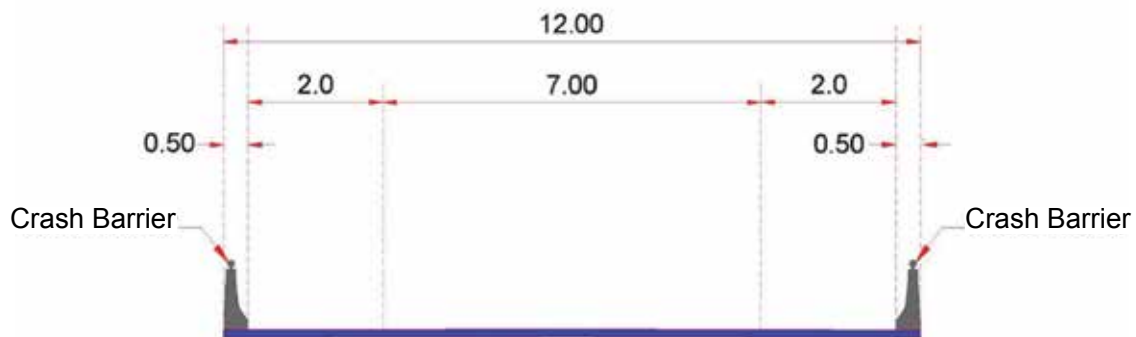
Fig 7.10 Typical cross section of grade separated structure, 2-Lane Highway (Open country - all terrain)
