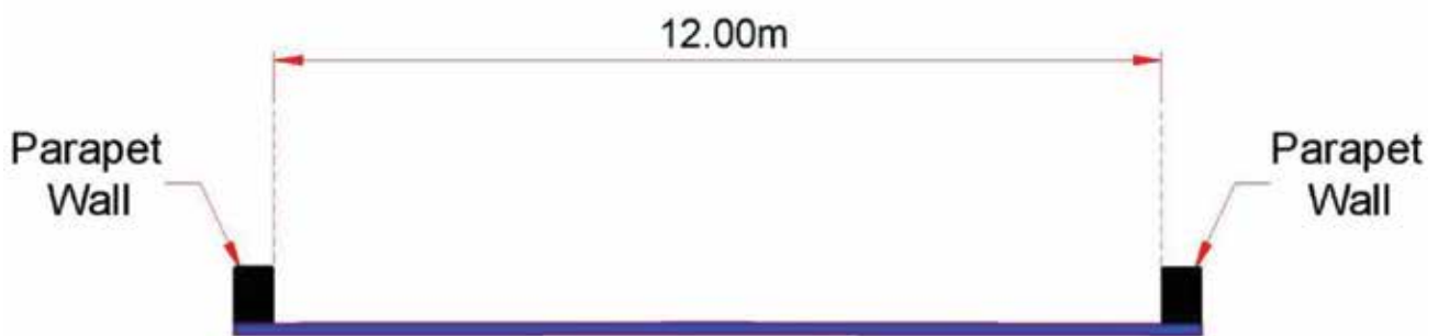
Fig 7.2 Typical cross section of Culvert at deck level for 2-Lane Highway without earthen shoulders (Open country - Plain/rolling terrain)
