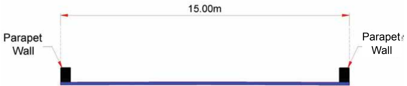
Fig 7.1 Typical cross section of Culvert at deck level for 2-Lane Highway (Open country - Plain/rolling terrain)
