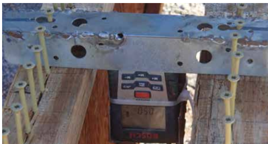
Fig. II-5 Positioning of Laser Distance Measuring Device for Profiling
