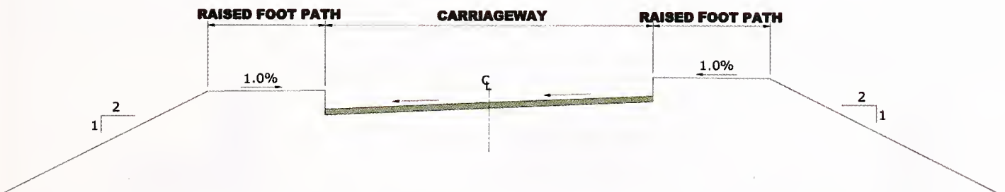
Fig. 4.8 A Typical Cross-Section of Road in Super-Elevated Section with Single Camber Provided In a Kerbed Carriageway (Urban Situation)
