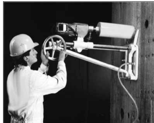
ii. Core Cutting in the Field
