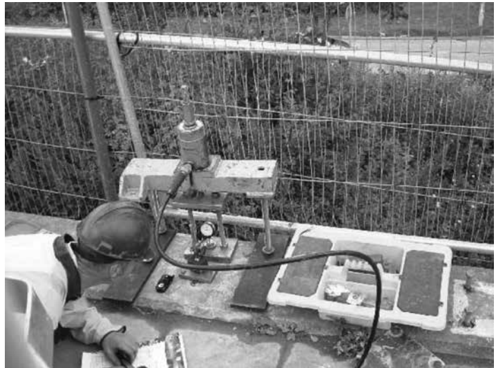
Fig. A25 Pull-Out Test
