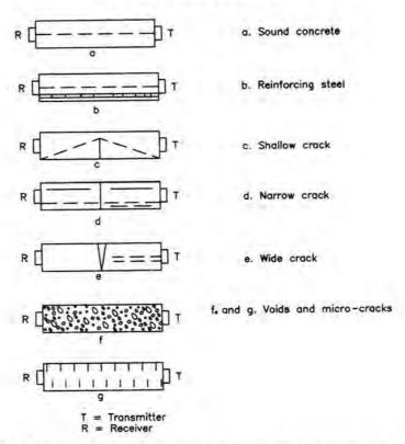
Fig. 3.8.2. Factors Affecting the Transmission of Sound Wave through Concrete<sup>8</sup>
