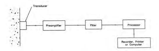
Fig. 3.9.1. Acoustic Emission Equipment 11
