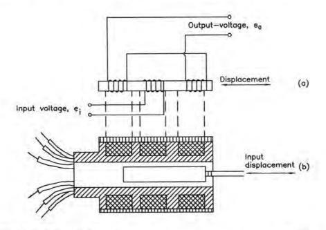
Fig. 3.24.1. Differential Transformer (a) Schematic Arrangement and (b) Section through a Typical Transformer <sup>99</sup>
