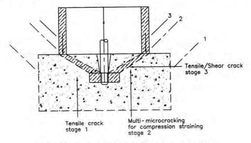
Fig. 3.4.3. Internal Cracking Stages during a Pull-out 153
