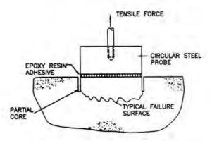
(b) Arrangement for testing partially cored specimens
