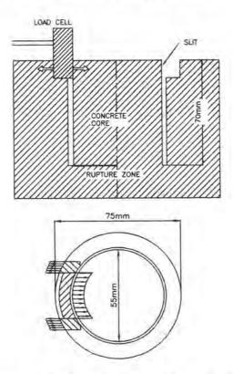
Fig. 3.6.1. Principle of Operation of the Break-off Test<sup>72</sup>
