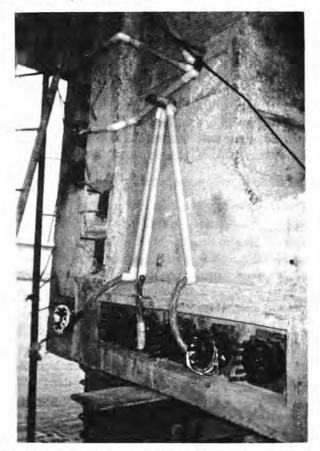
Fig. 3.38.1. Various Arrangements for Cable Resistance Measurements
