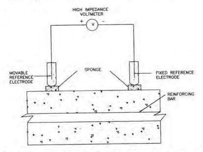
Fig. 3.32.1. Electrical Circuit showing Two Reference Electrodes used for Surface Potential Measurements
