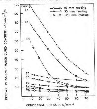
Fig 3.11.6. Influence of Concrete Grade on the Increase in ISA under various Curing Conditions with respect to Water Cured Concrete 80
