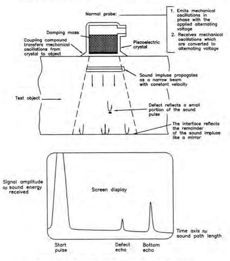
Fig. 3.10.1. Principle of Ultrasonic Examination<sup>87</sup>
