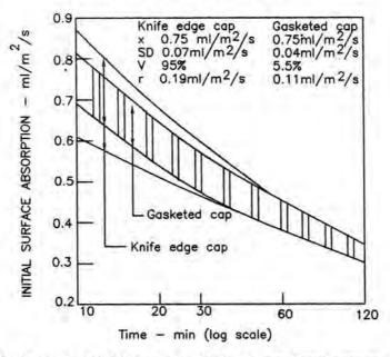
Fig. 3.11.4. Repeatability of ISA Test, 10 min. Values. Test Concrete: Water/Cement Ratio 0.55 Cured 3 Days in Water then in Air,
