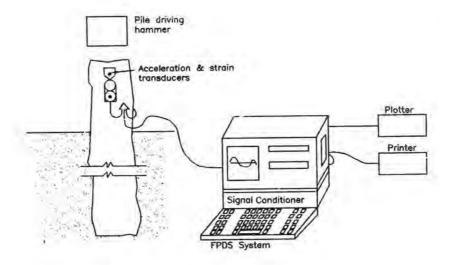
Fig. 3.39.4. System Concept for PDA/DLT<sup>157</sup>
