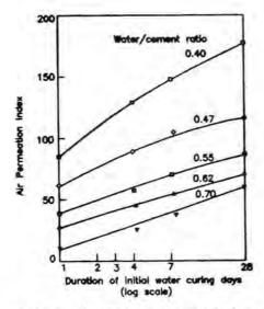
Fig. 3.12.3. Influence of Curing Conditions on Concrete Air Permeation Index, Modified Figg's Test, Test age 28 days<sup>80</sup>
