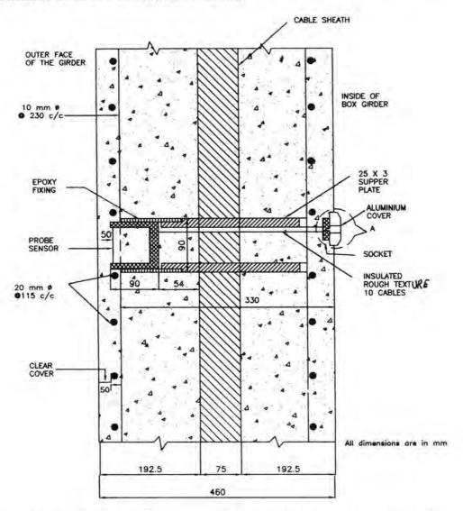
Fig. 3.37.1. Plan showing the Position of Corrosion Monitoring Probes and Sockets to be Installed in Web Portion of the Box Girder
