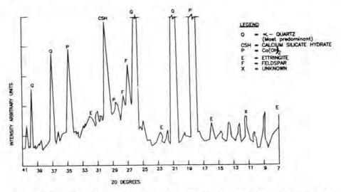
Fig. 3.17.1. X-ray Diffraction Pattern of an Old Hardened Concrete Sample
