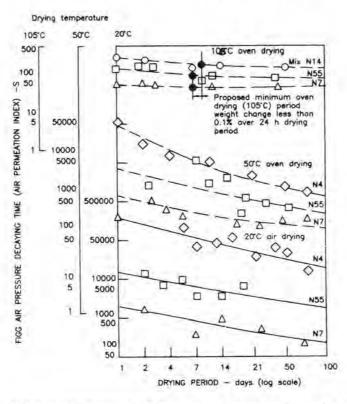
Fig. 3.12.2. Relationship between Air Permeation Index and Duration of Drying<sup>80</sup>
