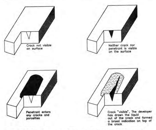
Fig. 3.18.1. Procedure used when Performing an Examination with a Penetrant<sup>87</sup>
