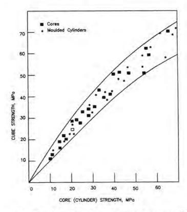
Fig. 3.3.1. Cube/Core (Cylinder) Strength Relationship<sup>3</sup>
