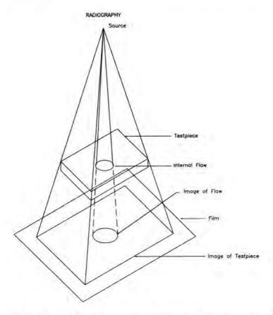
Fig. 3.19.1. Schematic Diagram showing Radiographic System 90
