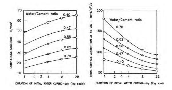
Fig. 3.11.5. Influence of Initial Moist Curing on Strength and ISA, Test Age 28 Days<sup>80</sup>
