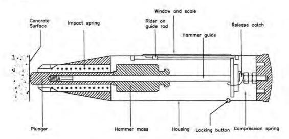
Fig. 3.1.1. Typical Rebound Hammer 11
