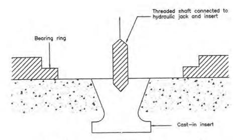
Fig. 3.5.1. North American Pull-out Method Assembly
