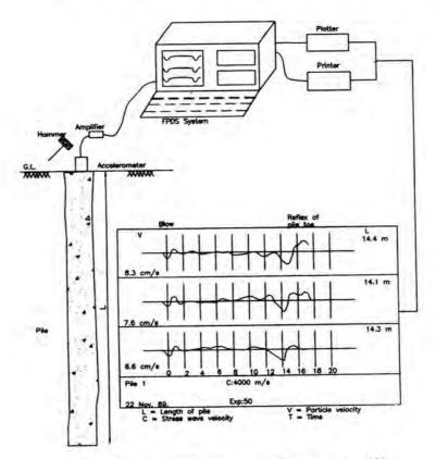
Fig. 3.39.1. System Concept of Integrity Test 158
