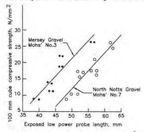
Fig. 3.2.2. Typical Low Power Calibration<sup>1</sup>
