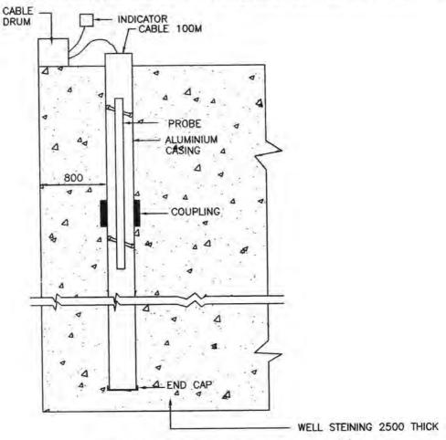
Fig. 3.28.1. Inclinometer System (Schematic) 169
