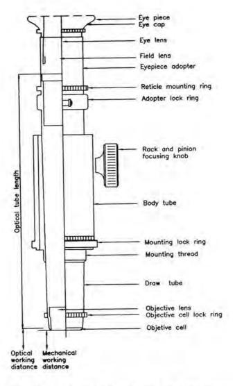
Fig. 3.20.1. Section through a Simple Low-Power Microscope 99
