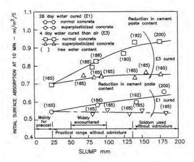
Fig. 3.11.7. Effects of Concrete Slump on its Initial Surface Absorption 80
