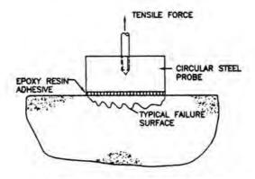
(a) Arrangement for testing uncored specimens
