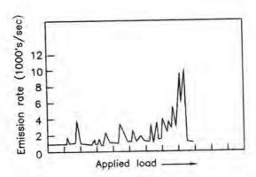
Fig. 3.9.2. Typical Acoustic Emission Plot<sup>11</sup>
