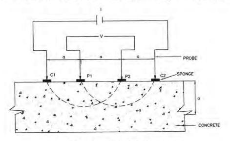
Fig. 3.36.1. Circuit of FPR Meter
