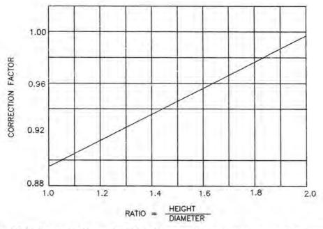
Fig. 3.3.2. Correction Factor for Height/Diameter Ratio of Core (as per IS:516-1959)
