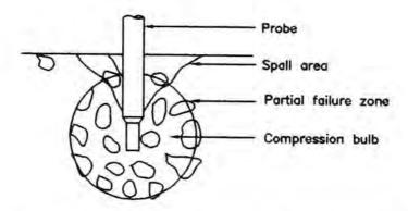
Fig. 3.2.1. Compression Bulb Produced by Penetration Probe1
