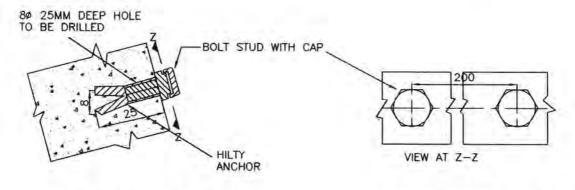
SECTION SHOWING FIXING OF BOLT STUDS FOR MECHANICAL GAUGE ALL DIMENSIONS ARE IN MM
