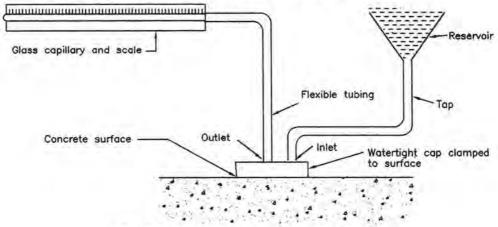
Fig. 3.11.1. Initial Surface Absorption Test<sup>11</sup>
