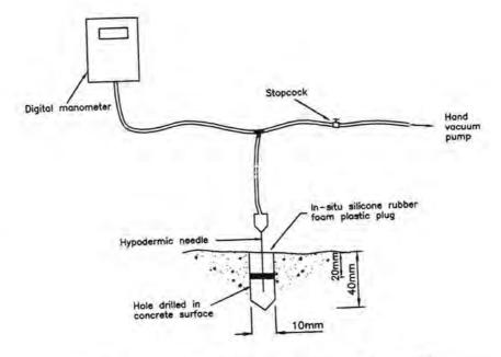
Fig. 3.12.1. Modified Figg's Air 'ermeability Test11
