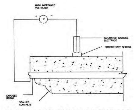
Fig. 3.31.1. Electrical Circuit for Open Circuit Potential Measurements
