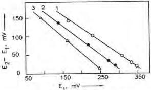
Fig. 3.22.2. Relation between E1 and (E2-E1) to get Rebar Dia (1) 6 mm Dia, (2) 10 mm Dia, and (3) 16 mm Dia<sup>5</sup>
