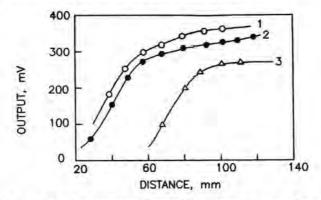
Fig. 3.22.1. Relation between Cover Thickness (distance in mm) with Output Voltage (mv)<sup>5</sup>
