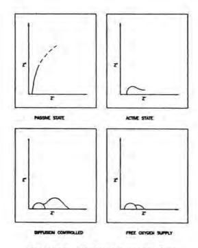
Fig. 3.34.3. Typical Impedance Plots
