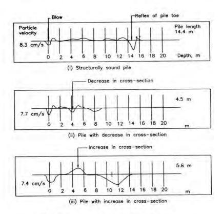
Fig. 3.39.3. Typical Integrity Test Results 155
