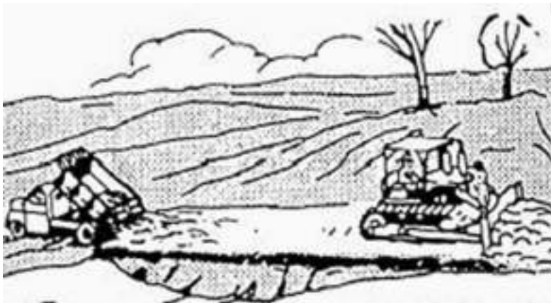
Fig. 28: Spreading by Dozer
