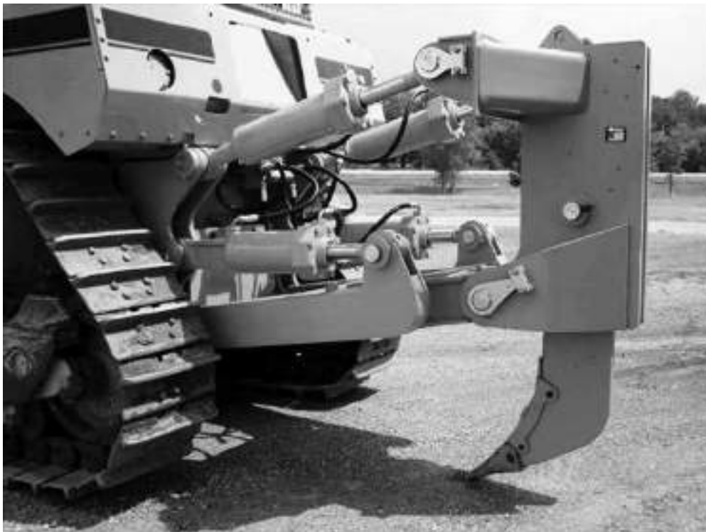
Fig. 19: Dozer with Ripper Attachment
