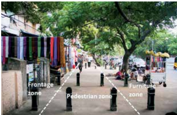
Photo 29: Well-designed footpaths have a clear, unobstructed pedestrian zone and a smooth walking surface: Besant Nagar, Chennai (left) and Aundh D P road, Pune (right).
