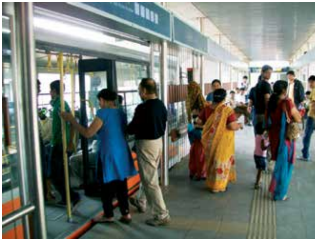
Photo 15: At-level boarding, demonstrated in Ahmedabad (left) and Lanzhou (right), makes boarding and alighting safe and easy, particularly for the elderly, disabled and people with special needs. It also improves system speeds by minimising the time taken for boarding and alighting.
