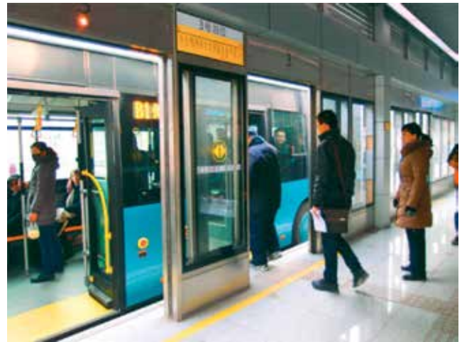
Photo 15: At-level boarding, demonstrated in Ahmedabad (left) and Lanzhou (right), makes boarding and alighting safe and easy, particularly for the elderly, disabled and people with special needs. It also improves system speeds by minimising the time taken for boarding and alighting.
