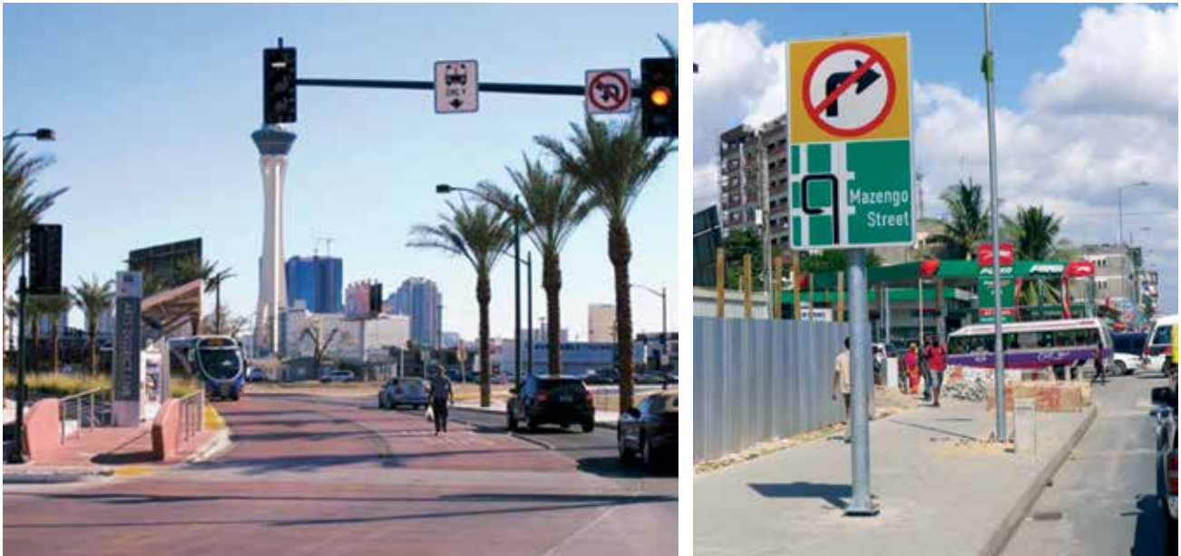
Photo 23: Forbidding turns across the bus lanes increases bus speeds at intersection: Las Vegas BRT (left) and DART BRT, Dar es Salaam (right).
