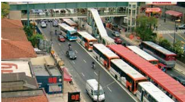
Photo 10: In Sao Paulo, high saturation levels at BRT stations can lead to bus queuing (left). In Jakarta, passengers experience delays due to high saturation levels at major terminals (right).
