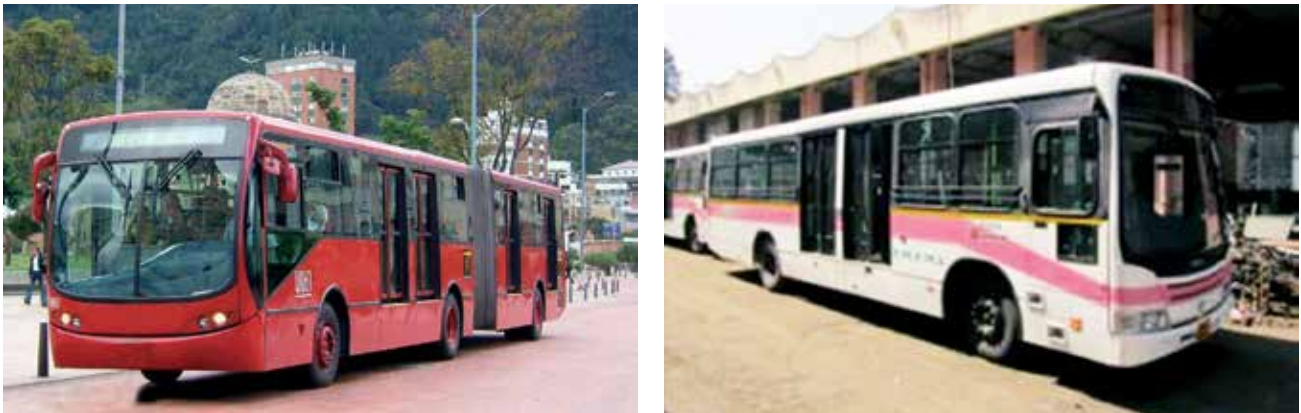
Photo 17: Wide doors on the station side of buses allow for fast boarding and alighting: 18m articulated bus in Transmilenio, Bogotá (left) and a 12 m bus in Rainbow, Pune (right).
