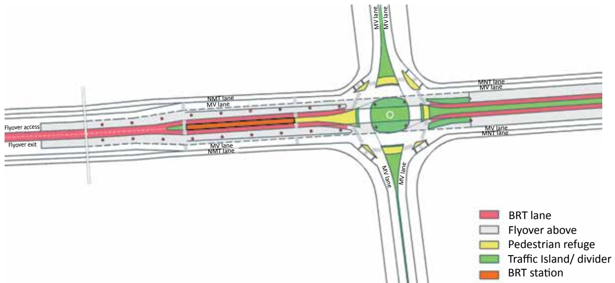
Fig. 28: Split flyovers can help maintaining the continuity of BRT lanes. Below the flyovers, stations are conveniently placed near the intersection and a square-about intersection design allows for a two-phase signal cycle.
