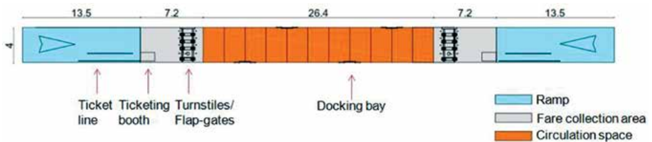
Fig. 12: Typical BRT station configuration incorporating ramp, fare collection area, and circulation space.
