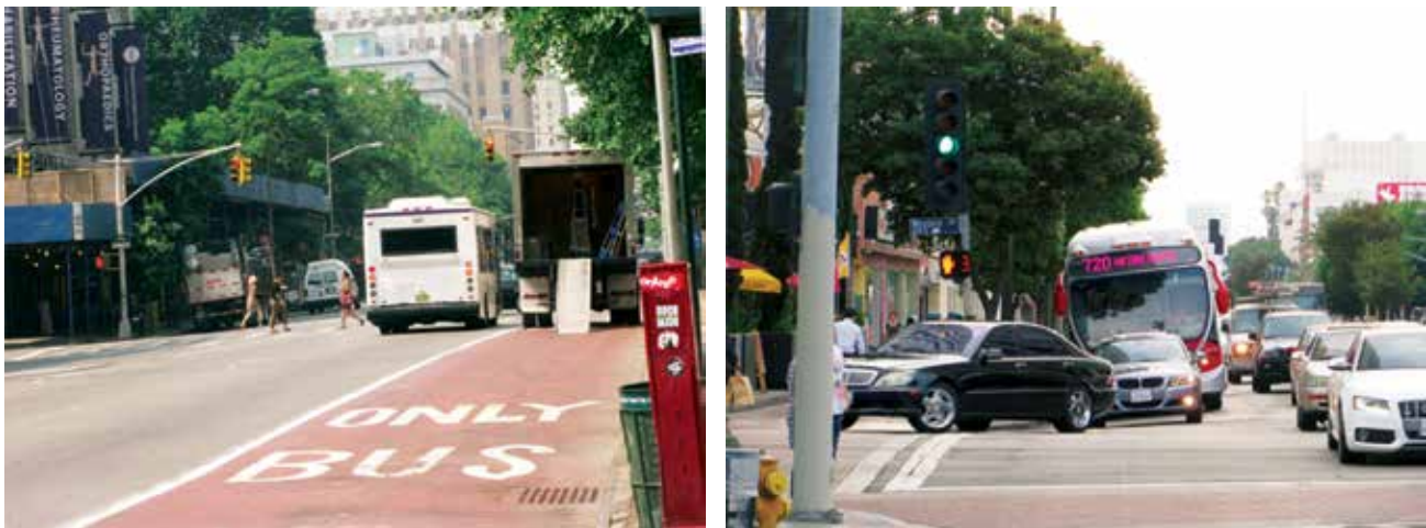
Photo 1: Parked vehicles and standing delivery trucks can compromise the utility of kerbside bus lanes (left): New York City, USA. Mixed traffic turning movements can also block kerbside lanes, leading to slower bus speeds (right): Los Angeles, USA.
