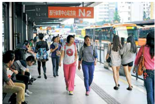
Photo 19: The BRT stations should offer seating, leaning bars, and adequate circulation space to meet expected passenger demand: Rainbow, Pimpri-Chinchwad, India (left) and GZ BRT, Guangzhou, China (right).
