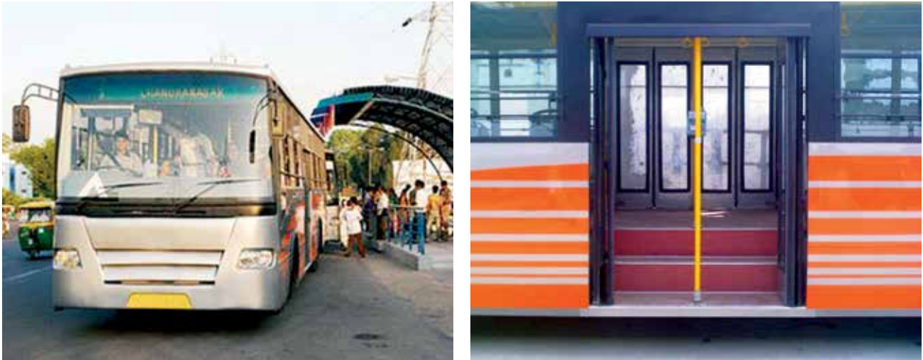
Photo 4: The Janmarg system (Ahmedabad, India) has doors on either side of the BRT bus to serve passengers in the corridor as well as in feeder areas. The high floor buses are not commuter friendly outside the corridor.
