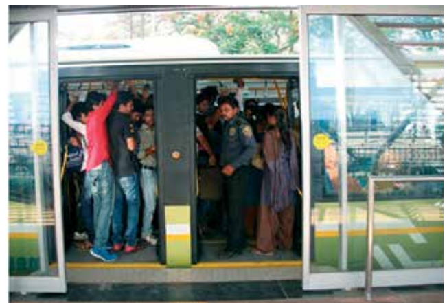
Photo 16: Sliding doors at stations improve as safety for passengers and prevent fare evasion: Rainbow BRT, Pimpri-Chinchwad(left) and iBus, Indore (right). (Photos courtesy: WRI India Sustainable Cities)
