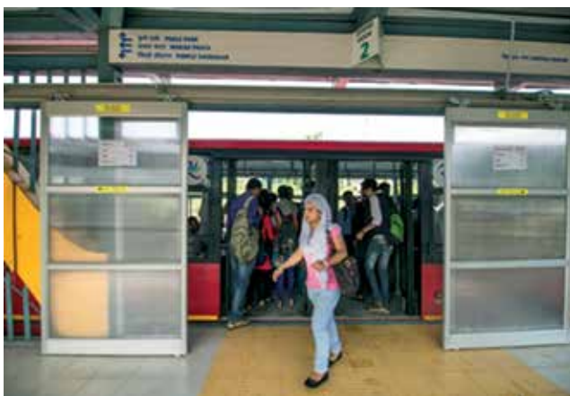
Photo 16: Sliding doors at stations improve as safety for passengers and prevent fare evasion: Rainbow BRT, Pimpri-Chinchwad(left) and iBus, Indore (right). (Photos courtesy: WRI India Sustainable Cities)
