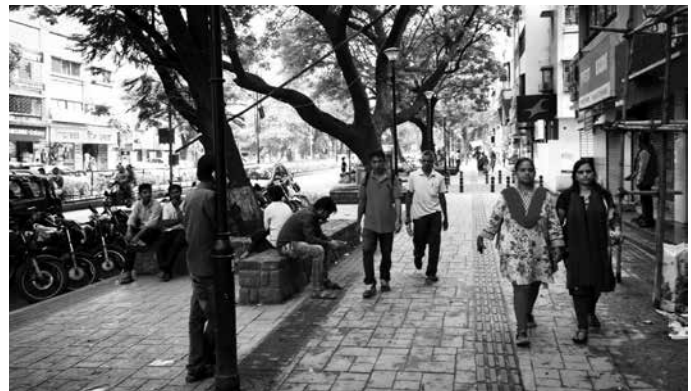
Photo 29: Well-designed footpaths have a clear, unobstructed pedestrian zone and a smooth walking surface: Besant Nagar, Chennai (left) and Aundh D P road, Pune (right).
