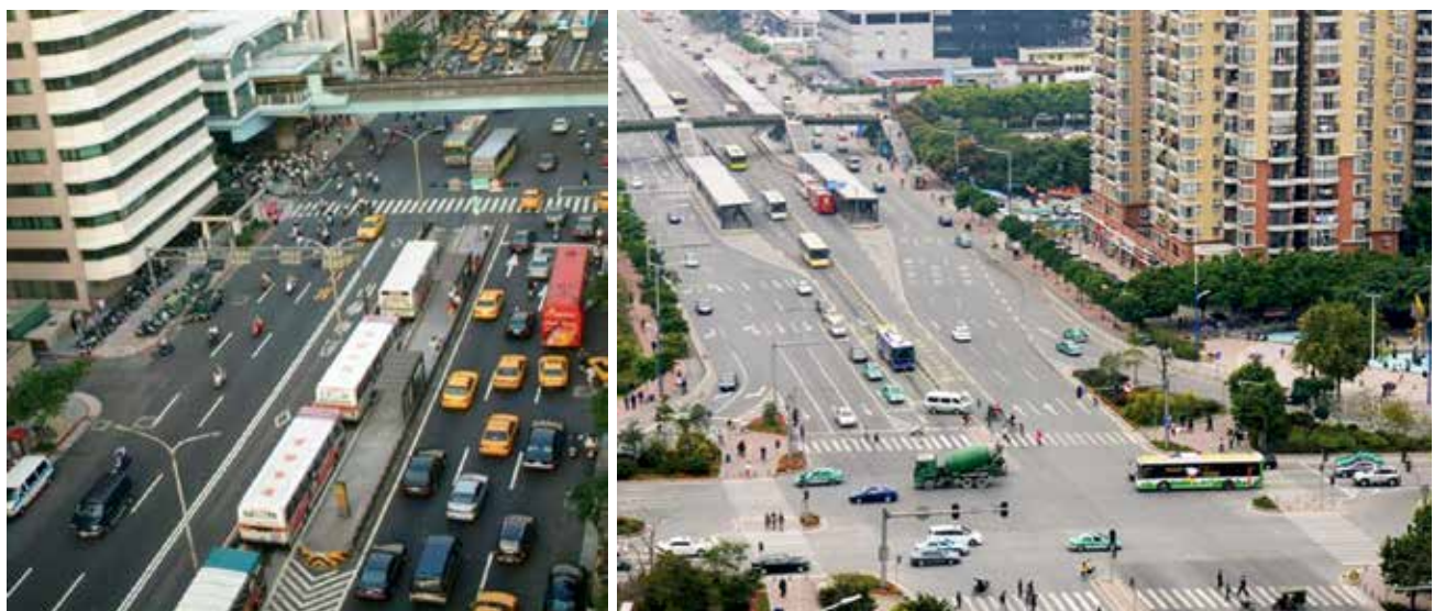
Photo 25: Left Image: Station placement exactly at the intersection results in operational inefficiency (Taipei, Taiwan). Right image: Station set-back from the intersection allows buses to queue at the intersection without blocking the docking bays (Guangzhou, China).
