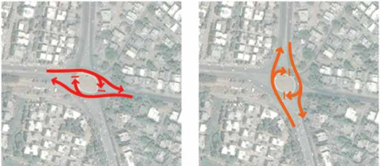
Fig. 23: Signal phases for a signalised roundabout (squareabout) intersection.
