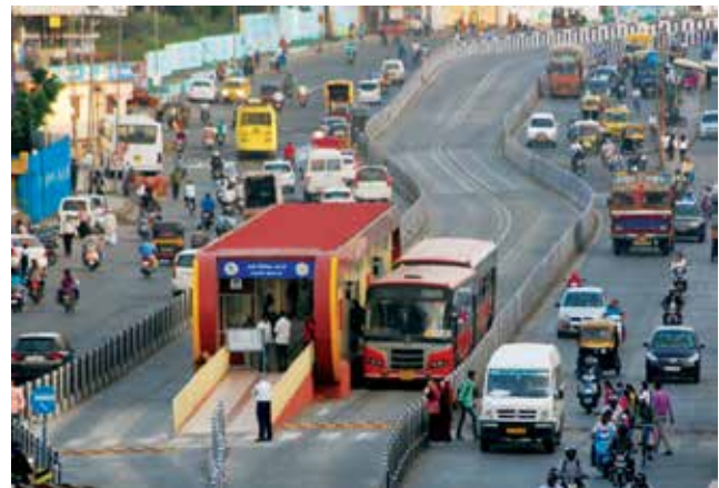
Photo 7: Median busway alignment avoids conflicts with other traffic, especially from turning movements from mix-traffic lanes: Ecovia, Quito, Ecuador (left) and Rainbow, Pune (right).
