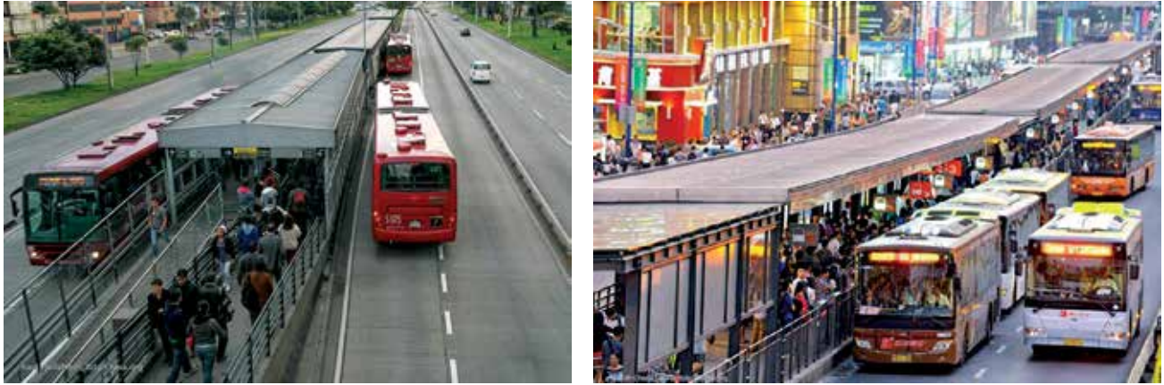
Photo 11: Multiple sub stops increases the capacity inside the station: Transmilenio, Bogotá (left) and Guangzhou BRT (right).
