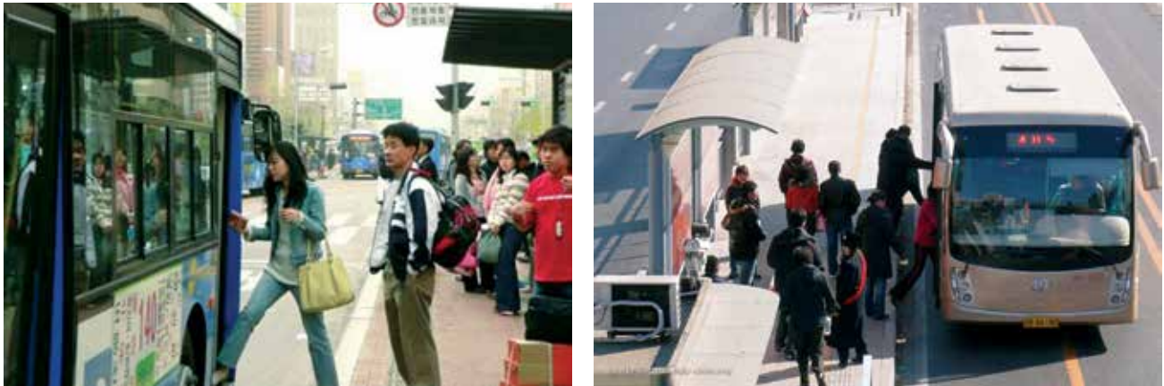
Photo 2: A lack of level boarding and on-board fare collection in Seoul, South Korea (left) and Dalian, China (right) leads to higher boarding times.
