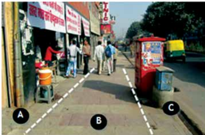
Photo 28: The three main zones of a footpath: (A) the frontage zone, (B) the pedestrian zone, and (C) the furniture zone
