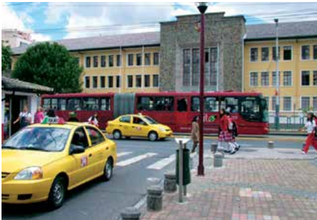
Photo 7: Median busway alignment avoids conflicts with other traffic, especially from turning movements from mix-traffic lanes: Ecovia, Quito, Ecuador (left) and Rainbow, Pune (right).
