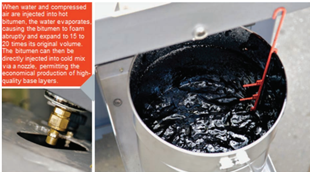
Laboratory scale foam bitumen plant
