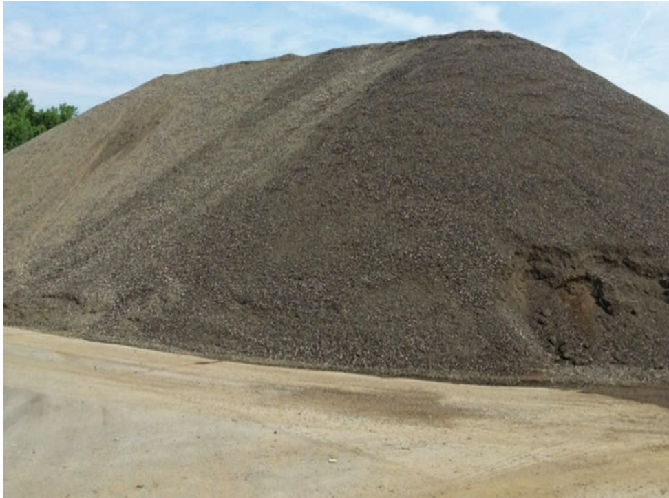
Asphalt material Reclaimed by Milling Machine
