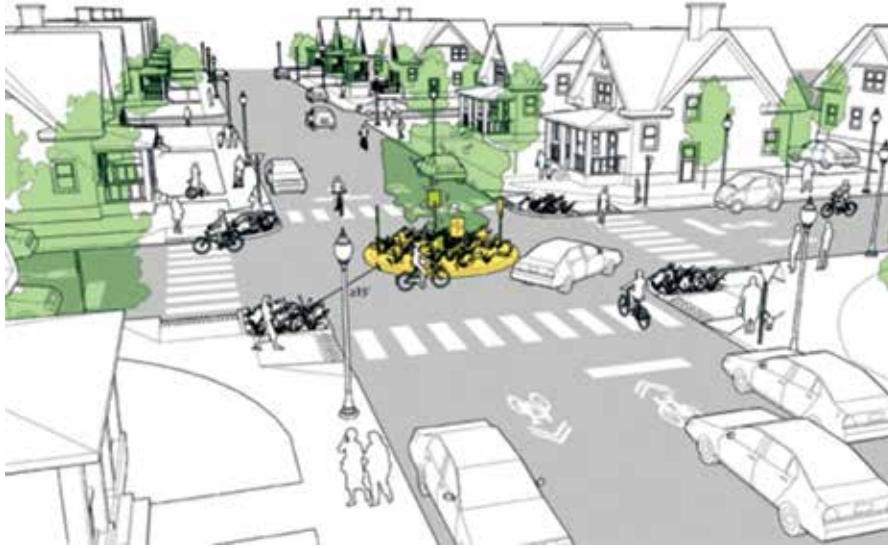
Fig. 2.14 Mini Roundabouts can be Useful in Slow Speed Urban Environments
