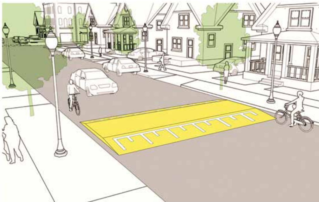
Fig. 2.5 Trapezoidal Hump – Flat Top with Tapered Sides
