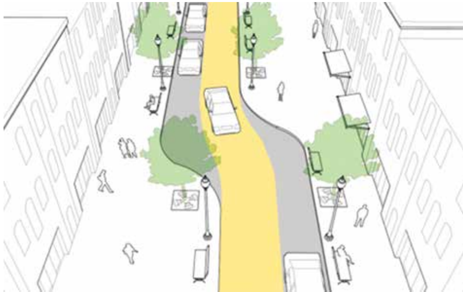
Fig. 2.18 Chicane is Another Design Element Used for Staggering
