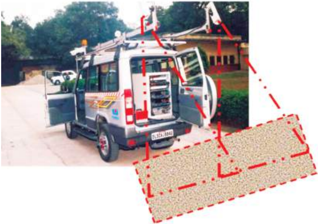
Photo 7 Pavement Surface Imaging Using Pavement Cameras
