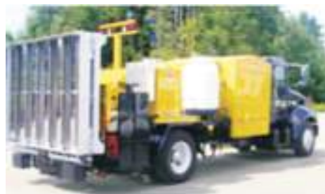
11.3 Infrared road patching technology
