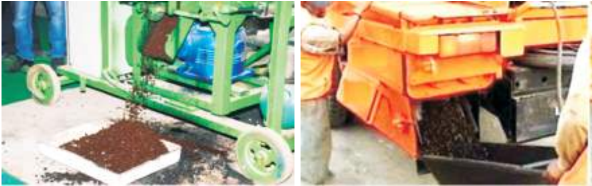
11.1 Production of Emulsified Cold Mix for Patching Mixes
