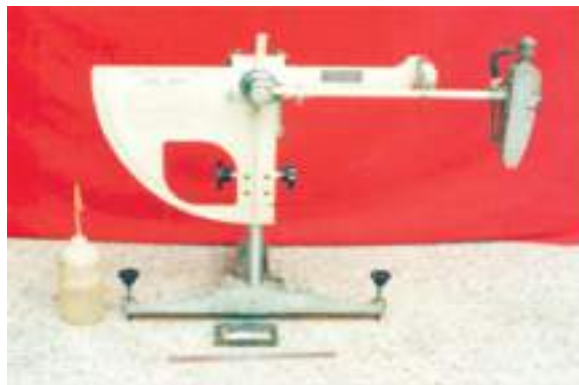
Photo 8 A Typical View of Portable Skid Resistance Tester
