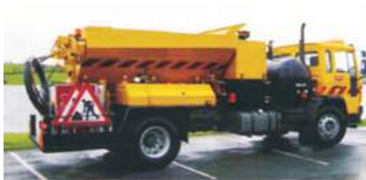
11.2 Velocity Injection Jetpatching Machine
