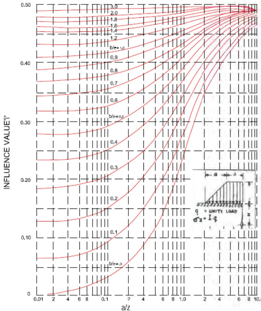
Fig. 4.3 Influence Chart for Vertical Stress Embankment Loading Infinite Extent Boussinesq Case
