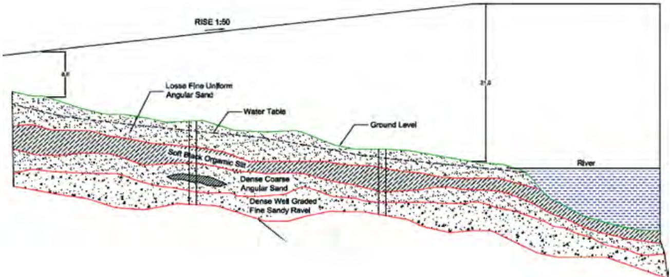
Fig. 2.3 Longitudinal Profile of the Subsoil
