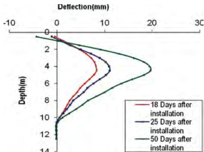
Fig. 6.10 Typical Incliner Output
