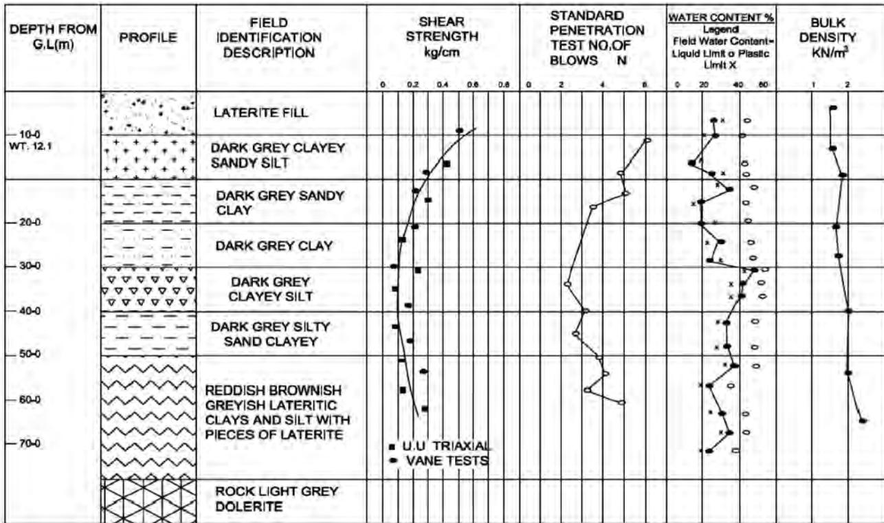
Fig. 2.4 Boring log and Summary of Sub-Soil Properties
