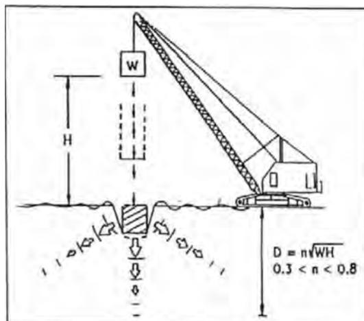
Fig. 5.3 Systematic Arrangement of Dynamic Compaction
