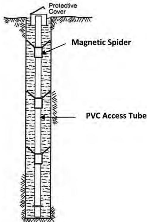
Fig. 6.7 Parts of Magnetic Settlement Gauge
