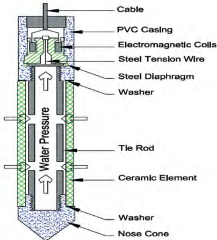
Fig. 6.4 Vibrating Wire Piezometer
