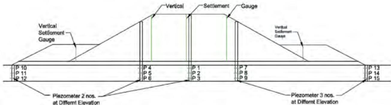
Fig. 6.11 Typical Cross Section of Earth Embankment with Instrumentation
