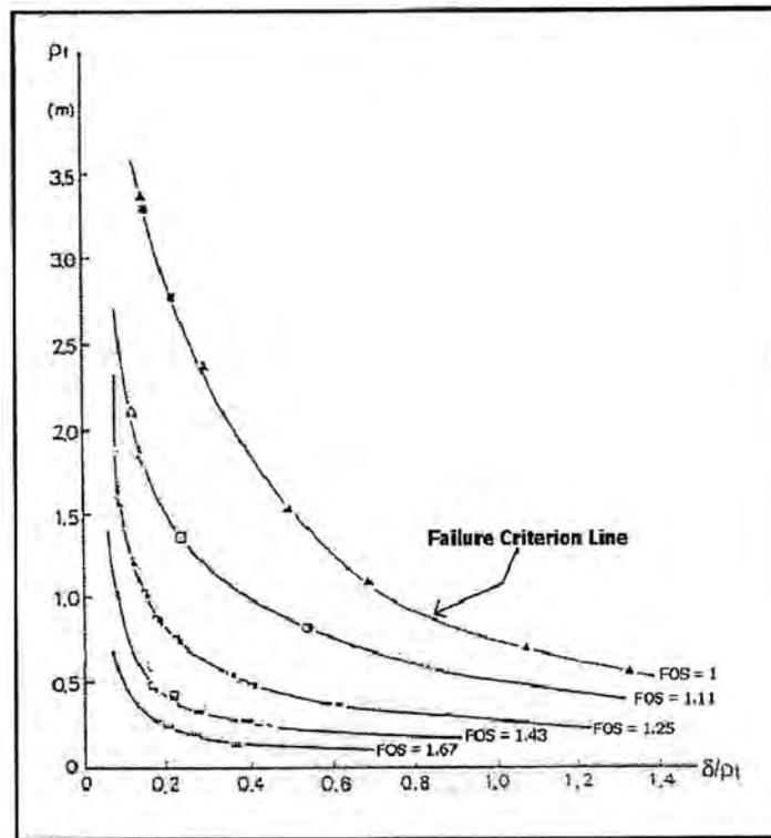
Fig. 6.15 Minoru Matsuo Embankment Stability Diagram
