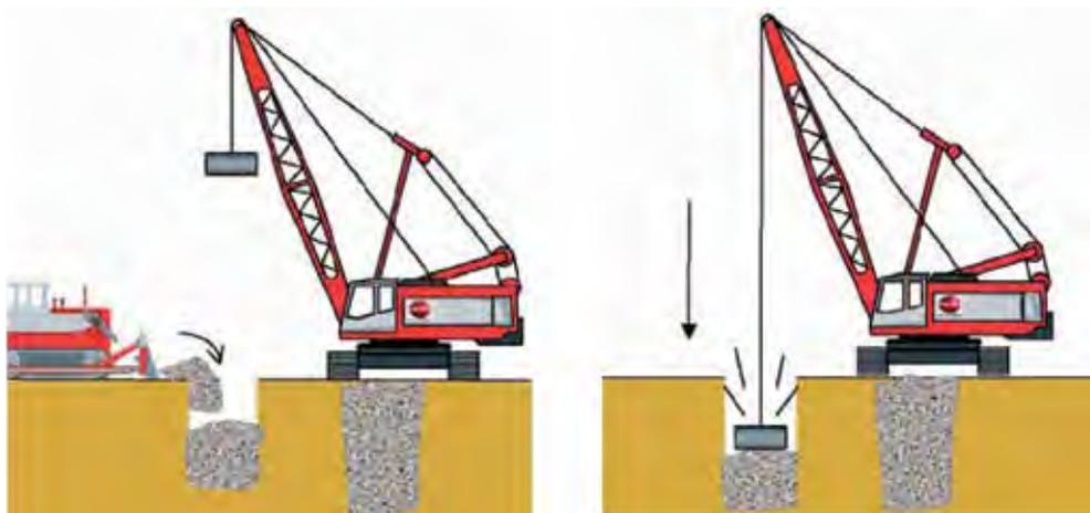
Fig 5.5 Construction Sequence Dynamic Replacement
