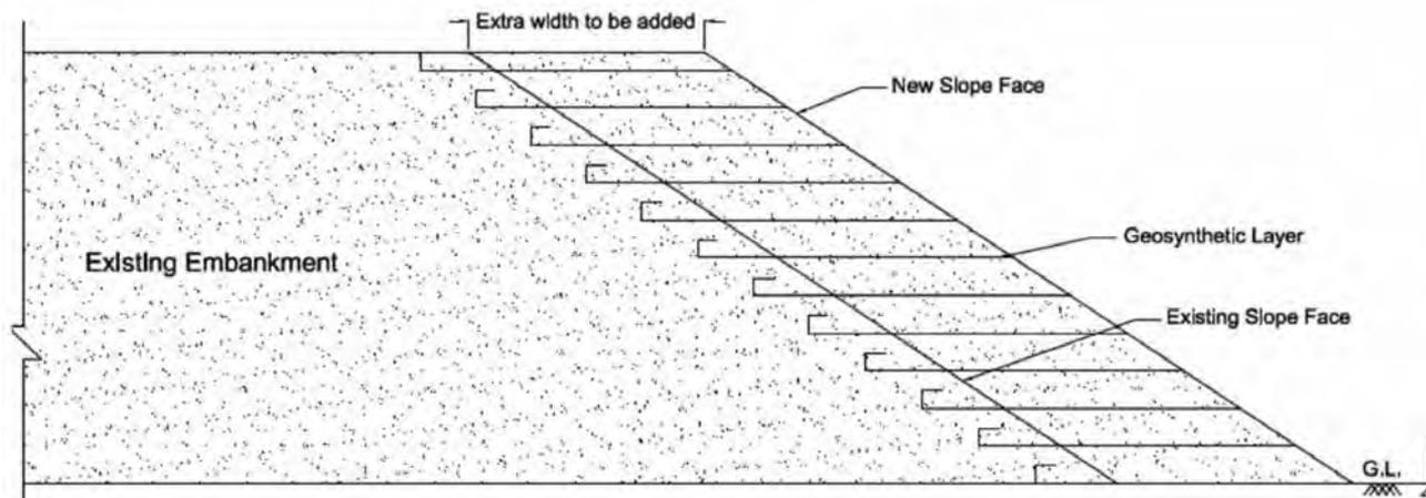
Fig. 8 (a) Widening of Embankment by cutting Benches and Filling
