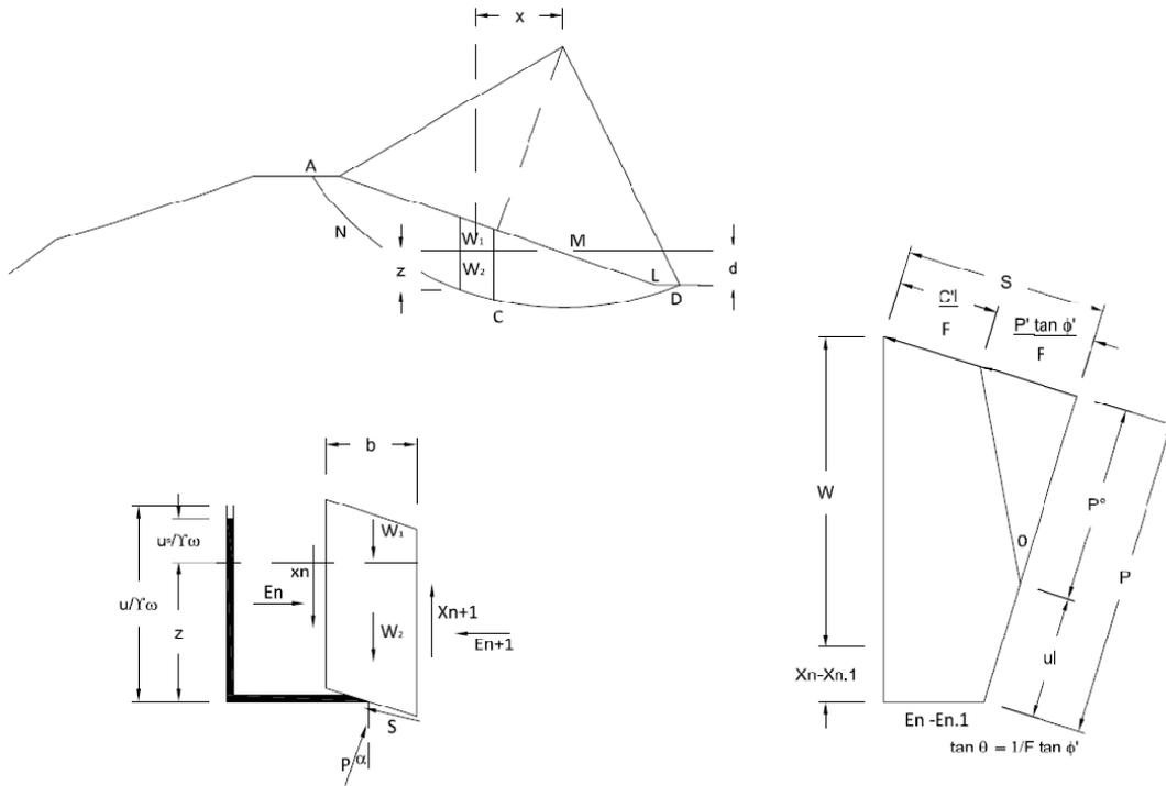
Fig. 3.6 Stability Analysis of Partially Submerged Slope by Bishop's Routine Method
