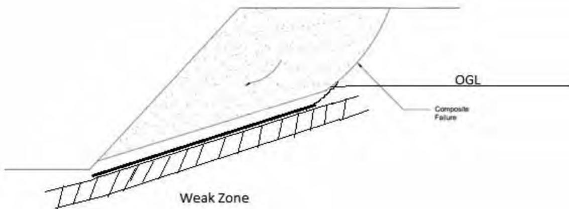
Fig. 3.1.b Composite Failures along non Circular Surface
