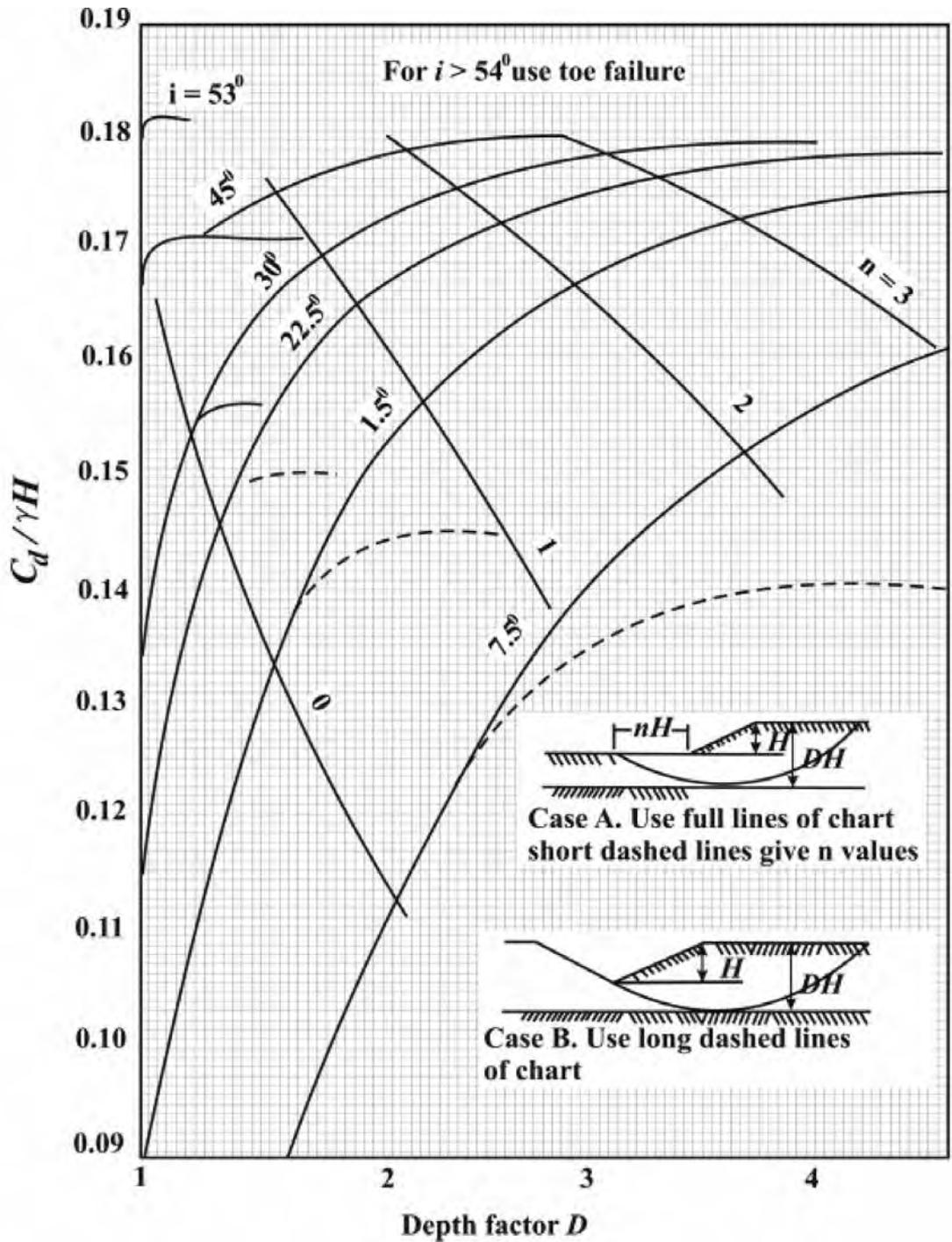
Fig. 3.3 Chart of Stability Numbers for the Case of Zero Friction Angle and Limited Depth
