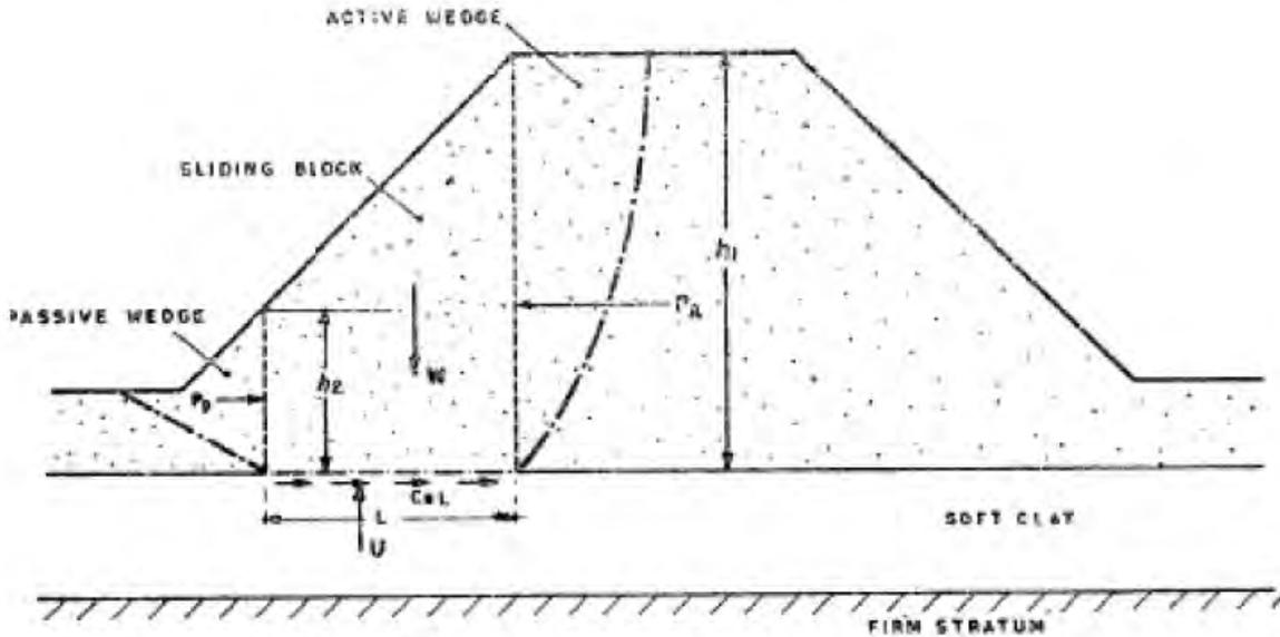
Fig. 3.8 Sliding Block Analysis
