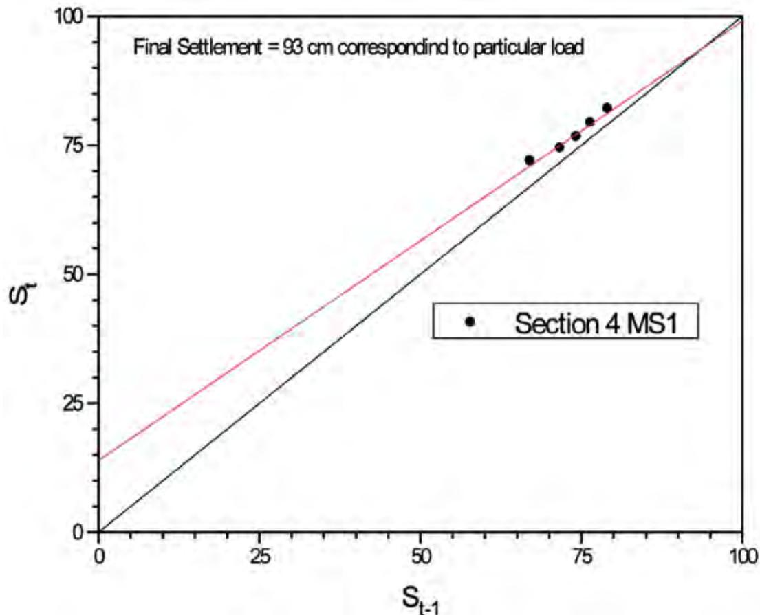
Fig. 3.14 Predicting Final Settlement Using Asaoka Method
