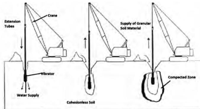
Fig. 5.4 Vibro Compaction Process
