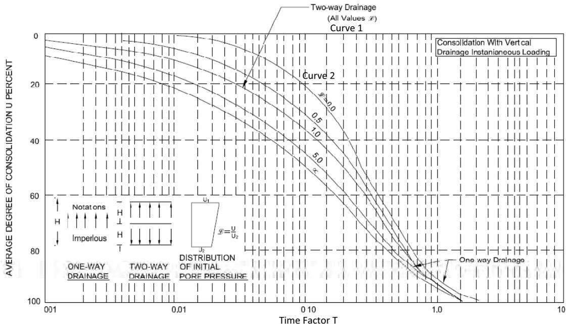
Fig. 4.2 Time Factors for Consolidation Analysis
