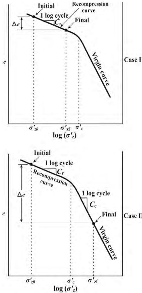
Fig. 4.1 Consolidation of Over-consolidated Soil
