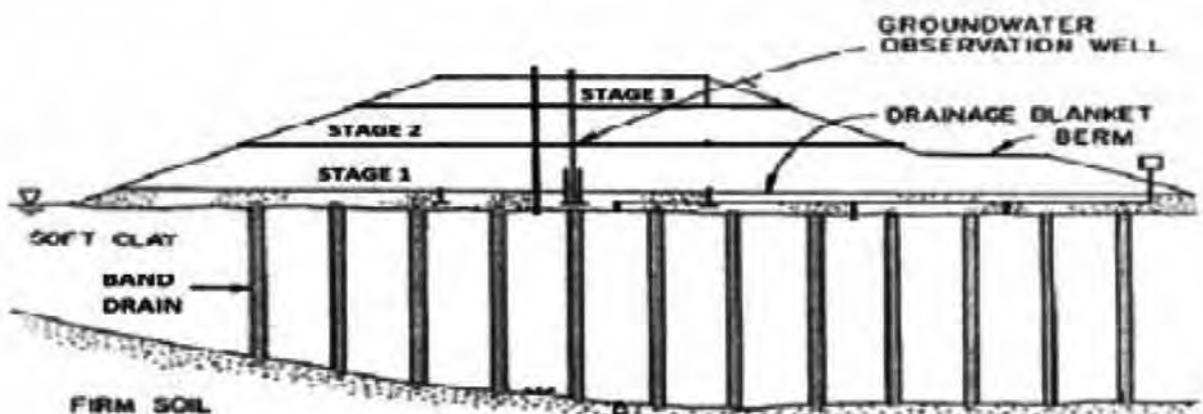
Fig. 5.1 Typical Cross Section of PVD Installation for Embankments
