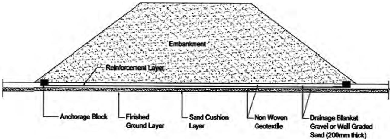
Fig. 5.6 Basal Reinforced Embankments (for more details, refer IRC:113)
