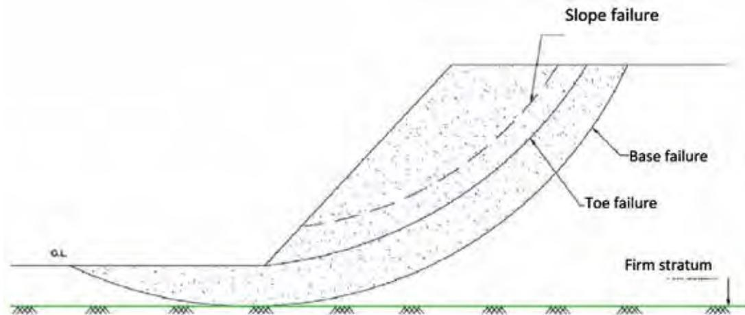
Fig. 3.1.a Rotational Failure Along Circular Surface
