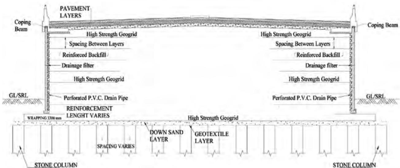
Fig. 5.7 Pile supported Basal Reinforced Embankment
