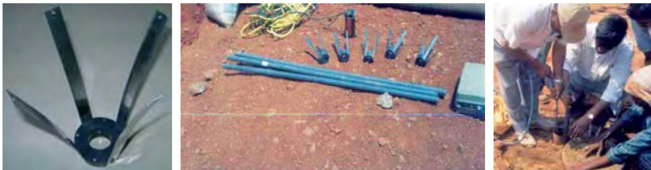
Fig. 6.6 Magnetic Spider, PVC Access Tubes and Installation of Magnetic Settlement Gauge
