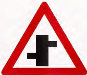
Fig. 15.21 Staggered Intersection
