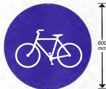
Fig. 14.52 Compulsory Cycle Track/Cycle Only
