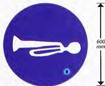
Fig. 14.57 Compulsory Sound Horn
